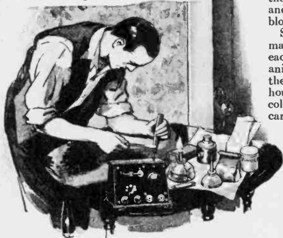
How a dent or crack is filled by melting a shellac stick into it, just as sealing wax is applied. Only a few inexpensive materials are needed for touching up all ordinary types of furniture scars
