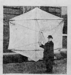
A scene at St. John's, Newfoundland, showing Senatore Marconi's arrangement for using a kite to support the antenna which he used in his first experiments. (Left) The kite itself.
