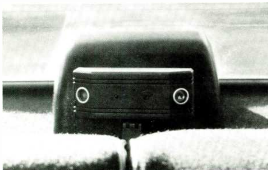
Mount the ultrasonic sensor in passenger compartment. If your auto has a brake light in the rear window, the brake light housing provides excellent cover.
