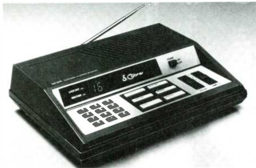
The Cobra SR-900, which offers coverage from 29 to 54 MHz, 136 to 174 MHz, and 406 to 512 MHz, is fully keyboard-programmable, and features a priority channel, instant NOAA weather selection, individual-channel lockouts, automatic 3-second scan delay, 4-hour memory protection, 16-channel scan memory, manual channel access, and a large LED display.
