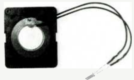
This piezoelectric disc has been connected to an NE2 neon lamp. Rap the disc, and the lamp will flash.
