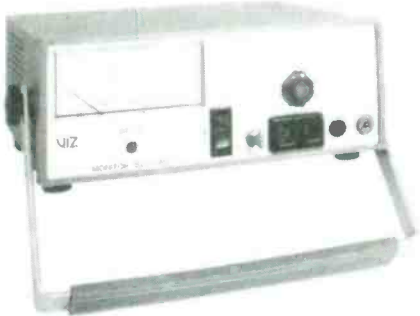
This professional isolator allows a technician to select the output voltage for the device under test.
