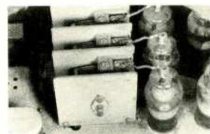
This view of the Gloritone's chassis shows the 24-A screen-grid tubes wired to the three-section tuning condenser. The power transformer, with its ventilating cover, is seen just to the left of the tuning condenser.
