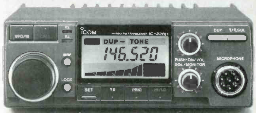
ICOM's IC-228A (25 watt) and IC-228H (45 watt) scanners may be programmed for twenty memory channels, and features a priority channel, lock-outs, search/scan, and an optional tone-squelch module. Unit transmits on 2-meter band.
