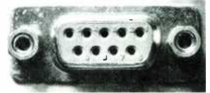
Follow the numbers embossed on the D-connectors. Don't count pins or guess—the male and female connectors are mirror images, so it's easy to get confused.
