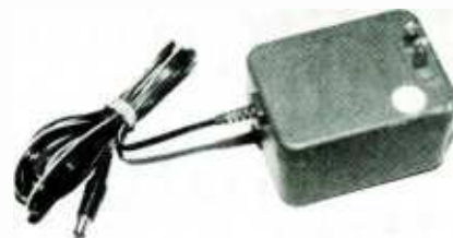
A wall-mounted power supply capable of providing between 8 and 24-volts DC at 1 amp can be used to power the Print Buffer/Spooler. The author chose a 9-volt unit as his power source.
