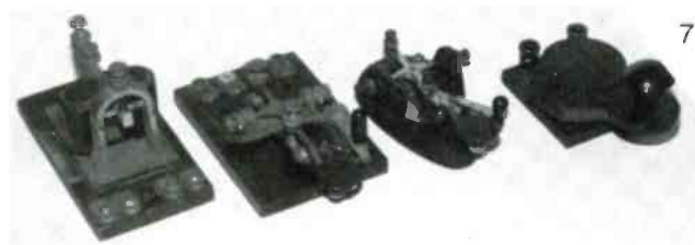
For the CW operator! The sounder and key on the left are from the wire-telegraph days. A McElroy and a J-5 flameproof are on the right. You can hook these up today.
