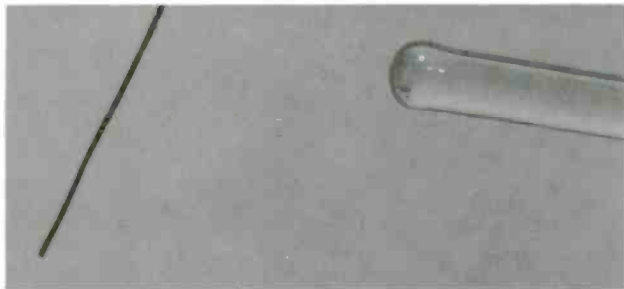
The positive charge on a glass rod repels the positive charge on silk thread. Positive charging results from depleting a material of its electrons.
