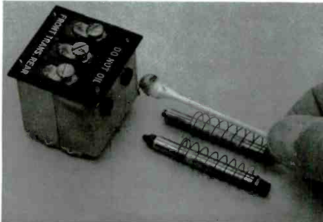
Use a cotton Q-tip dipped in cleaner to remove goo from the plunger tubes. But be certain not to oil the tubes nor the plungers (not even a drop), or use an oil-based cleaner.
