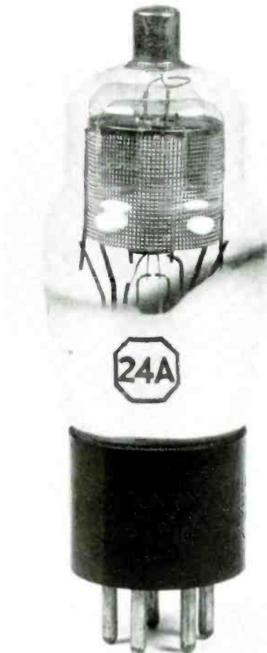
Type 24A tetrode vacuum tube was most common screen-grid device used in consumer radios in the early '30's. Originally released with a pear-shaped envelope, it was changed to the "ST" style shown here a few years later.
