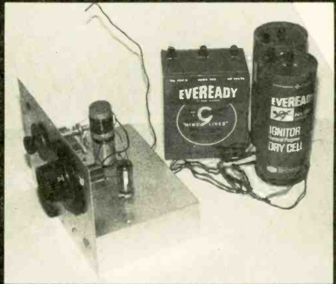
Here's a one tube shortwave receiver designed by the ARRL for the Boy Scouts. It's still good for code practice.
