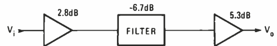
Fig. 5—Gain computations are not more complex for circuits containing filters. A filter's gain is simply negative for a given signal. Subtracting the loss from the gain gives you the overall gain or loss figure.
