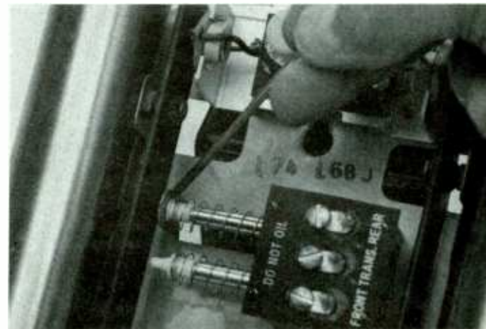
A metal stop prevents the rear-door plunger from ever striking the second tone bar, thus you hear one tone.
