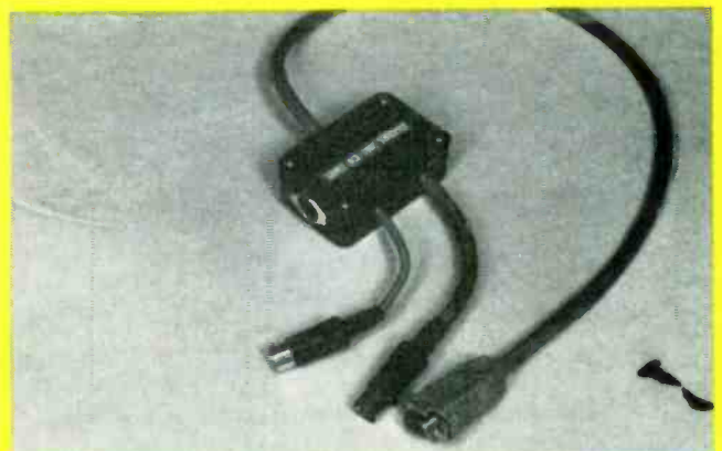
The Sanyo RGB Sync Inverter is built into a small plastic box. The Sanyo keyboard cable plugs into the box jack, another plugs into the computer RGB output, and the long cable connects to the RGB monitor input cable.
