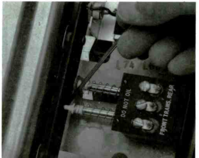
The pointer shows how the back of the front-door plunger rests against a tone bar. That is the position it returns to in order to make the second “bong” sound.
