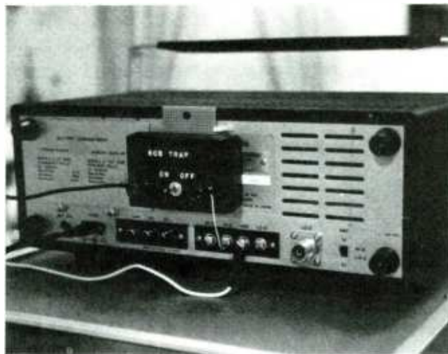
The assembled BCB Trap is connected between the antenna system and the receiver, with the receiver's connecting wire kept short. Here it is mounted on the back of the author's receiver.
