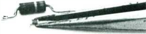
The small black speck at the tip of the tweezers is a surface-mounting resistor. As shown, you can convert a conventional 1/4-watt resistor into a surface-mounting type like the SMT by shaping the axial leads downward.
