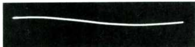
Here is a photo taken from an oscilloscope of the ripple on the 9-volt power source indicating good voltage regulation with variation less than a small fraction of a percent.
