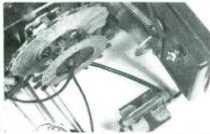
This close-up shows some of the components that make up the set: Honeycomb-wound coils (top left); hinged-plate variable capacitor (top right) with a spring that holds the plates apart and rod-mounted cam that forces them together. Capacitor with clip-mounted grid-leak resistor is at bottom.
