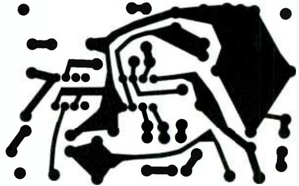
Fig. 4—The circuit board can be constructed using this foil pattern as a guide. Be sure to trim the solder pads as shown so that they do not interfere with other traces.
