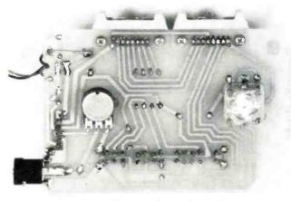
As you can see the tuning capacitor and potentiometer are mounted on the foil side of the board. Note also how the contact strips on the coaxial connector hold it in place.
