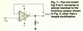
shown in Fig. 7 may be used. The load-current equation for the non-inverting version remains unchanged except for the polarity:
