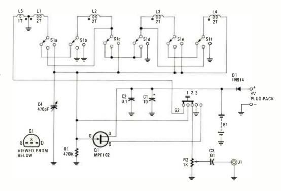
Fig. 2—The circuit uses a FET buffer amplifier (Q1) to provide amplification with high input impedance. The output level control R2 can be used to adjust the output gain so as not to strain your radios AGC on large signals. Inductor L5 is a single turn (per layer of cable) which is used to provide a low-impedance output in the passive-loop mode. The loop is tuned by C4 which is a polycon variable capacitor.
