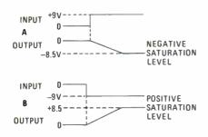
Fig. 12—Of course the output of an integrator can't reach infinity no matter how long the input signal is left on. The output is limited by the negative (A) and positive (B) power-supply values. A perpetual motion machine it's not.
