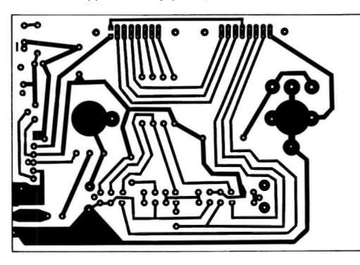
Fig. 3—The circuit-trace pattern shown here is the same size as the circuit board, so you can use this to make your own printed-circuit board using the positive resist method.
