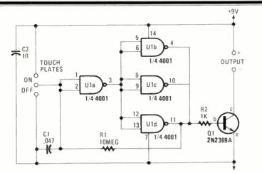
Fig. 2—This Touch Switch (which will control 9-volt DC loads of up to 100mA) is built around a 4001 quad NOR gate. U1b to U1d along with U1a form a bistable multivibrator. Touching the two upper contacts causes Q1 to conduct, pulling its collector low; thereby, completing a path to ground through the load circuit.
