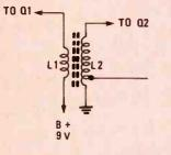
Fig. 2—Coils L1 and L2 are wound on a ½-inch diameter ferrite rod which may be cut to size from a longer rod. Mark a groove around the rod with a hacksaw or file and it will snap in two when tapped. Refer to text for coil winding information.
