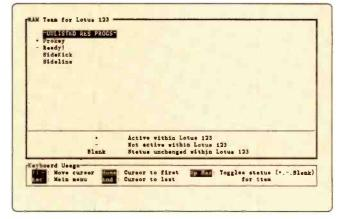
Fig. 2—RAM teams are those RAM-resident programs you would want to use with a particular program. Here, the RAM Team for Lotus 123 are + Prokey, -Ready, Sidekick, and Sideline. The + sign means that the program will be activated; minus, deactivate; and no sign means that the status will remain unchanged. For more information circle no. 81 on Free Information Card.
