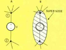
Fig. 5—A constant voltage source provides ACNAP with a way of computing the value of one node voltage by knowing another. That simplifies the matrix and speeds up analysis.
