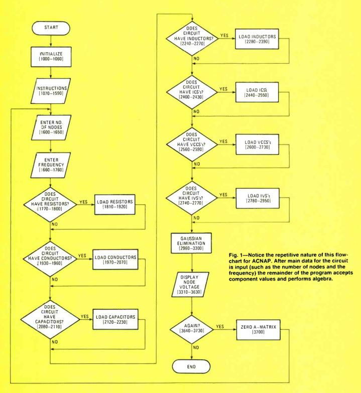
the value and the node connections of resistors, conductors, capacitors, and inductors. Beginning on line 3870, Input Subroutine #2 is used for the power supply devices, returning the node connections as well as the real and imaginary components (VR and VI, respectively) of the energy that those devices deliver to the circuit.
