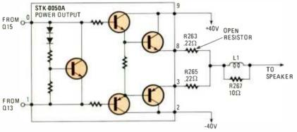
After locating an open or leaky transistor or IC, check each bias resistor. It's best to check bias resistors while the suspected transistor is out of the circuit. Often, the shorted
