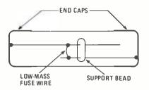
Fig. 4—This is one method of construction used to build a fuse with very-fast blowing characteristics in a 3AG case.
