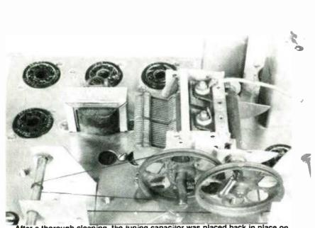
After a thorough cleaning, the tuning capacitor was placed back in place on the chassis. Note that one of the two dial cord systems has been restrung.
