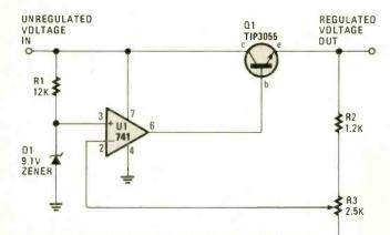
Fig. 1—In this basic voltage-regulator circuit, U1 (a 741 op-amp) serves as a reference voltage source—set by zener diode D1 and resistor R1—to control drive current to the base of Q1 (which is set up in a series-pass configuration).
