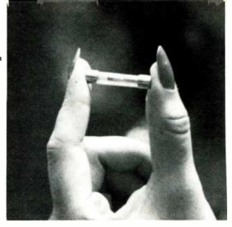
berylium/copper/silver-plated clips and holders is a must if the currents are above 5 amps. Heating at the fuseholder because of poor contact with the fuse will shorten fuse life. Be sure to remove the fuse from the holder when soldering the wires to the holder to avoid unnecessary heating of the fuse itself.
