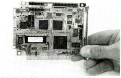
This half-size "WX-1" hard-disk controller has two smaller header terminal strips, which can each drive a disk drive. The larger header strip is split by a Y-adapter or a two-connector cable when using two disk drives.
