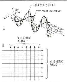
Fig. 1—Radio and TV waves are electromagnetic (EM) waves exactly like light, infrared, and ultraviolet, consisting of two mutually perpendicular oscillating fields (electric and magnetic, shown in "A"). If (as shown in "B"), at a great distance from the center, we take a look at a small slice of the advancing wavefront, we would be able to observe the electric and magnetic field vectors at right angles to each other. would be horizontally polarized.
