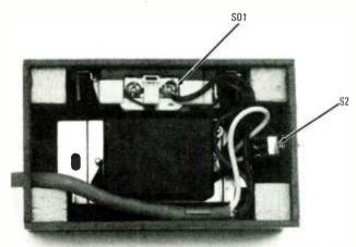
The prototype was built in an old light-dimmer case, but could easily have been built on perf- or printed-circuit board.
