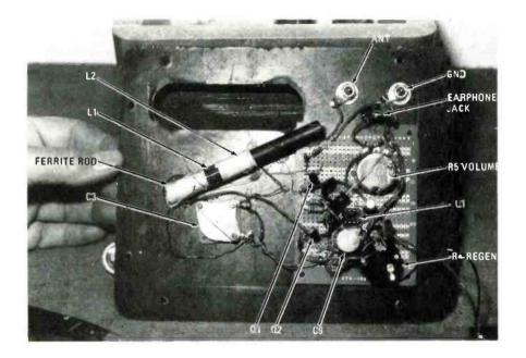
perfboard so both controls will fit flush with the top panel. Refer to the photos and Fig. 3. The shaft mounting nuts on the two controls will hold the PC perfboard to the front panel.
