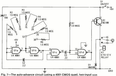
Fig. 7—The auto-advance circuit (using a 4001 CMOS quad, two-input NOR gate configured as inverters) advances the slides at intervals of 5, 10, 15, 20, 25 or 30 seconds, depending on the setting of switch S2.
