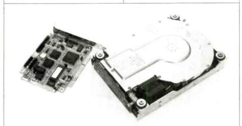
A hard disk system consists of a controller and a hard disk drive. This pair cost less than \$100. But notice the drive came without a front panel.
