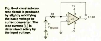
The input voltage is a stable DC reference voltage source (shown as a battery in the diagram). As with the conversion circuits discussed above, the load current  $(I_L)$  is determined solely by the input voltage  $(V_{in})$  and resistor R1 (R<sub>L</sub> has no affect) and is given by:
