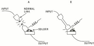
Fig. 5—A dual-action, slow-blow fuse blows in one of two modes: either the link melts under short-circuit conditions (A), or the solder blob melts due to continuous overload.
