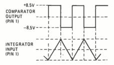
Fig. 16---The output waves from your home-brew function generator should line up like this, with the outputs varying between + 8.5 and -8.5 volts. Note the identical frequency.
