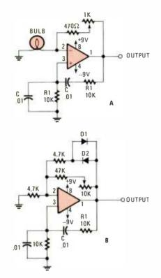
Fig. 17—If you can't get the light bulb needed for the circuit in A, then you can use the circuit in B. Its output will not be as clean, but is good enough here.
