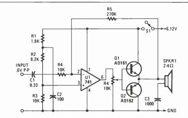
Fig. 1—The input signal is fed to the inverting input of U1 (a 741 op-amp, set up as an amplifier/buffer). U1's output is fed to the common-base leads of Q1 and Q2 (which you'll surely recognize as a push-pull amplifier). The input to the push-pull (feeding SPKR1) is controlled by R4, which serves as a volume control.
