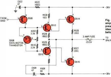
printed-circuit trace or poorly soldered connection may cause an imbalance in the amplifier's output at the speaker terminal. Sometimes, the voltage may leak through a good transistor, causing operating voltage to be only a few volts lower than normal. Double check the wiring with the lowresistance scale of the DMM.
