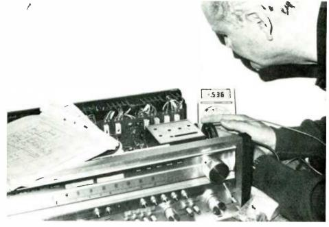
the capacitor is still "loaded," you may damage the meter. I once slapped my digital multimeter (set to read resistance) across a resistor that was near a charged filter capacitor. And what I ended up with is an expensive continuity checker -need I say more?
