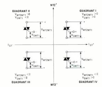
Fig. 3—Usually, triacs have their gates referenced to the main terminal (MT1) and all conduct when the voltage between MT1 and the gate reaches about 0.9 to 1.4-volts (positive or negative) depending on whether the triac operates in quadrant I or quadrant III respectively. Four-mode triacs also operate in two additional quadrants: quadrant II and quadrant IV.
