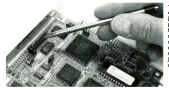
The pointer indicates one of several sets of jumper pins used to program the controller for specific drive characteristics. The controller usually comes with a data sheet that gives the jumper setting for most drive models.
