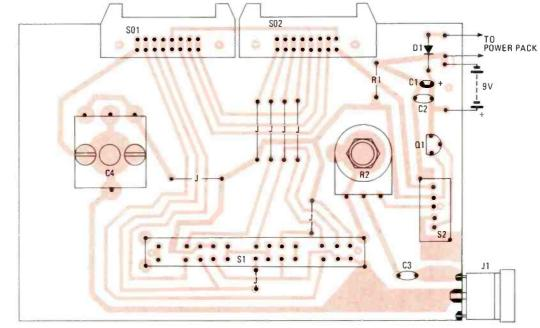
Fig. 4—Please take note that in this layout for the PCB, the tuning capacitor and potentiometer are mounted on the reverse (copper) side of the board.
