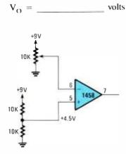
Fig. 13—In this comparator circuit, the non-inverting input is used to receive the reference voltage, and the inverting input as the signal being tested.
