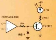
output is +8.5 volts, the transistor turns on lighting the LED. When the comparator output is -8.5 volts, the transistor is cut-off, therefore, the LED does not light. The transistor can be any common NPN unit. A silicon diode of any kind protects the transistor.
