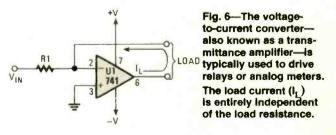
The circuit in Fig. 6 uses the inverting input, so the signal polarity is reversed. If that's undesirable in your particular application, the non-inverting, voltage-to-current converter
