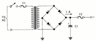
Fig. 3—A medium-acting fuse is used as F2 to provide faster action, while a slow-blow fuse is used as F1 because of the surge current provided to C1 at turn on.
