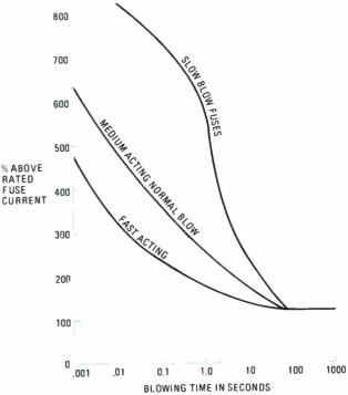
Fig. 2—Sometimes circuits are designed to run "hotter" than they are supposed to for certain applications. For that reason slow-acting fuses are needed since they tolerate overdrawn current for a length of time.
