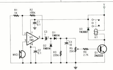
Fig. 3—The op-amp output at pin 6 is rectified by diodes D1 and D2, filtered by capacitors C3 and C4. The resulting DC output is applied to the base of transistor Q1, turning it Q1 on and, thus, the relay, activating the load.
