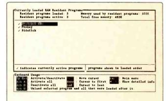
Fig. 1—Referee lets you look at currently-loaded RAM-resident programs. The screen image shows all the resident programs in the order in which they were loaded. Notice that descriptive names as well as file nomenclature appear. Referee lets you designate a descriptive name for each program in place of its filename—it's up to you.
