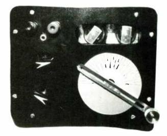
If antique knobs are not available, make some of your own. The round dial assembly was made from a piece of plastic with lines drawn through with a small soldering iron. Two coats of silver metallic spray paint makes it appear like a metal dial.
