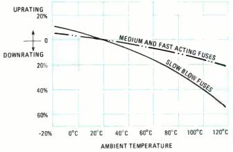
Fig. 1—A most important yet over looked characteristic of fuse operation is the ambient temperature. As you can see, as the temperature increases the rating of a fuse drops.
