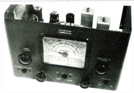
A frontal view of the reassembled Echophone. The top panel (containing the speaker) won't be replaced until the set is operating and needs no adjustment.
