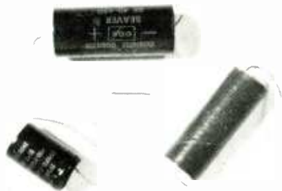
Replacement capacitors with any desired capacity can be created by connecting several individual units in parallel.
