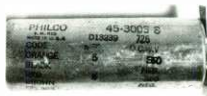
Carefully study the wiring information on the unit to be replaced; it's usually plainly marked. If the chassis does not reflect the capacitor orientation, mark it accordingly before removing the bad component, so that the replacement can be installed in the same way.
