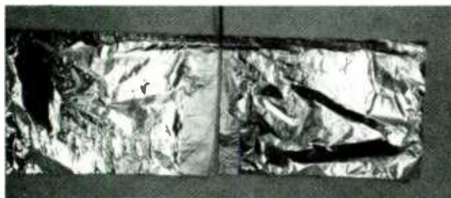
This FM antenna is shown mounted on a wall, but it could just as well have been mounted on a single 2 × 4 or light wood stripping for ease of mobility and adjustment.
