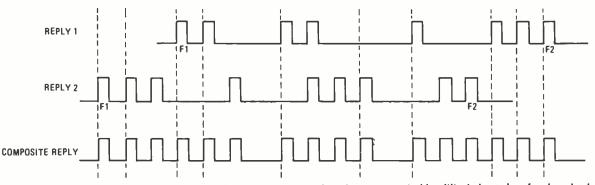
Fig. 12—Garbling is an example of what can happen when two aircraft are separated in altitude by only a few hundred feet, while being equal distances from the airport. The reply signals from the two craft are interlaced, producing a composite of the two replies.
