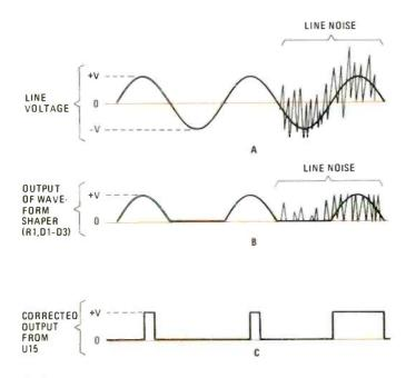
Fig 3—This graph illustrates the sequence of events that must take place in order for the TTL Clock to accurately keep time.
