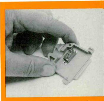
Install a subminiature DPDT slide switch on one half of a D-connector's plastic hood. Be sure to allow for cable leads to fit around switch. Refer to the text.
