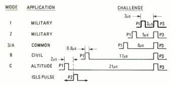
Fig. 3—This diagram gives the challenge modes generated by the coder circuits of the interrogator system, along with the uses for that mode. The mode of the transmission is determined by the time lapse between the leading edges of the P1 and P3 framing pulses. For instance, if the framing pulses are separated by 8  $\mu$ s, the transmission is mode 3/A, which is common to both civil and military use.
