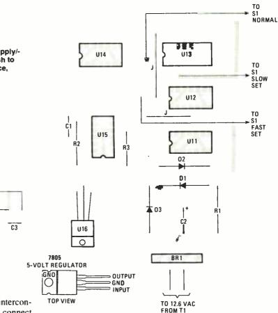
to SLOW to check for proper sequence of numbers. Check for proper timing by setting S1 to FAST; that should advance the display at a rate of 1 hour per second. (There should be 60 Hz at the FAST mode tap). In the SLOW mode, the display advances at rate of 1 minute per second (1 Hz). And in the NORMAL mode, the display's progression is at a rate of 1 count per minute (a frequency of 0.0167 Hz).
