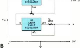
Fig. 3—Both the basic (A) and an extended version (B) of the constant-current setup is shown built around the LM317 positive, adjustable regulator. By using the LM317, most of the problems associated with using three-terminal regulators in constant-current applications can be eliminated.
