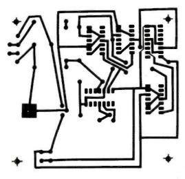
Fig. 6—Foil pattern of the power supply/frequency divider board. When mounting the diodes and electrolytic capacitor, be careful of their orientation.
