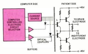
Fig. 5—The Dobelle device using monopolar, biphasic stimulation: A small electrode is applied to the cortical tissue, while a large indifferent electrode, placed under the scalp, is used for the return current.
