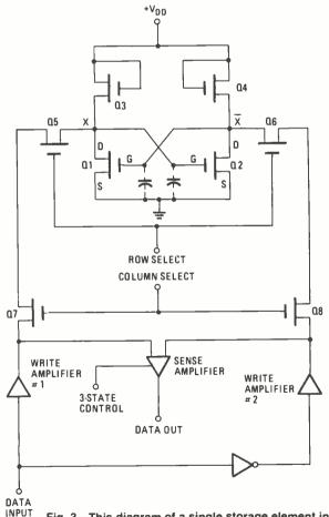
Fig. 3—This diagram of a single storage element in a static-memory chip illustrates the operation of each cell in the memory. In the static-memory cell, the storage element is a flip-flop.
