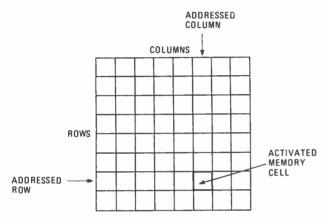
Fig. 4—Most semiconductor memories are organized in a matrix of storage cells. To access a particular cell, one row and one column must be activated.
