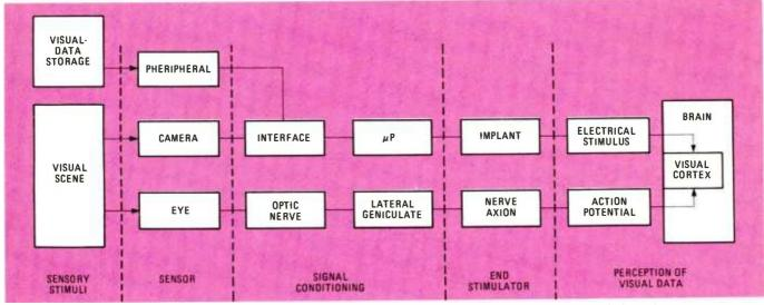
Fig. 3—A comparison between physiologically and artificially induced sight. Note the relationship between the various parts of the artificial vision system and its natural counterpart.
