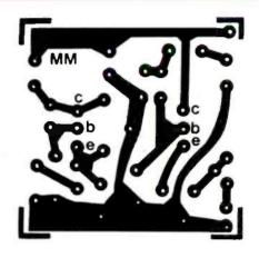
Fig. 2—The full-scale foil pattern shown may be lifted from the page and used to etch the printed-circuit board for the Magnetometer.
