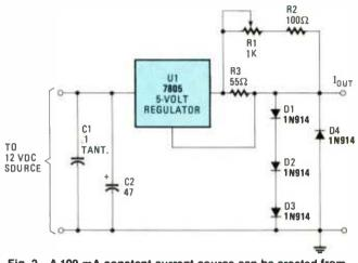
Fig. 2—A 100-mA constant current source can be created from a 7805, 5-volt regulator and a few additional components.
