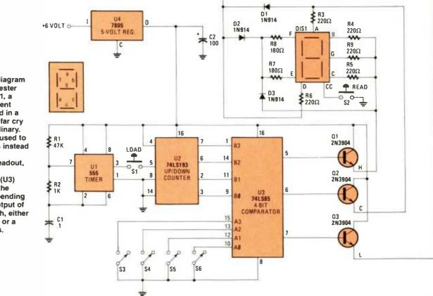
Fig. 1—The schematic diagram of the ESP tester shows DISP1, a seven-segment display, used in a way that's a far cry from the ordinary. That unit is used to show letters instead of the usual numerical readout, with a 4-bit comparator (U3) controlling the display. Depending on which output of U3 goes high, either an "L," "H," or a "C" appears.
