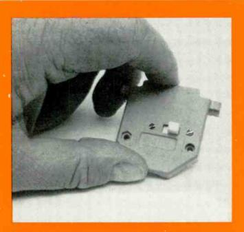
Make certain that the switch's handle is free to move to both extreme positions. If it's not, remove the switch and file the opening to accommodate the switch's handle travel.
