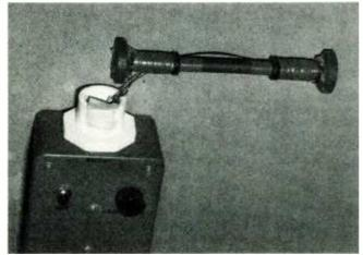
If you wish, the plastic pipe can be made longer so that the magnets will be farther from any ferroalloy on your person.
