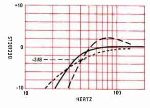
Fig.6—The solid curve shows the bass response of a critically designed, sealed enclosure. A too-small enclosure produces an undesirable peak (dashed), but too large causes the curve to droop (dotted).
