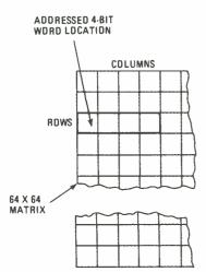
Fig. 8—The 2114, with its 1K  $\times$  4 configuration, can store 1024 4-bit words. The memory is arranged in a 64  $\times$  64 matrix, providing 4096 individual storage cells.
