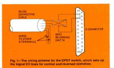
hood you will use as "the top." Pre-connect the switch's jumper wires before installing the switch in the hood. Make certain that you locate the switch as far to the rear of the hood as is possible and as close as possible to one side, so that the switch doesn't block the opening for the main cable. Also, double-check to make sure that the switch's handle can move its full length in both directions.
