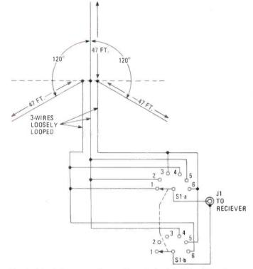
Fig. 2—The three-element Flexo installation provides greater flexibility over the two-wire type by allowing six combinations.
