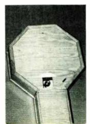
Every digital clock has a time-setting switch. The knob for S1 can be seen at the rear of the clock. Four positions provide a timeholding feature, a slow set where the time advances slowly, a fast set when the time advances rapidly, and a normal running position once the correct time has been achieved.
