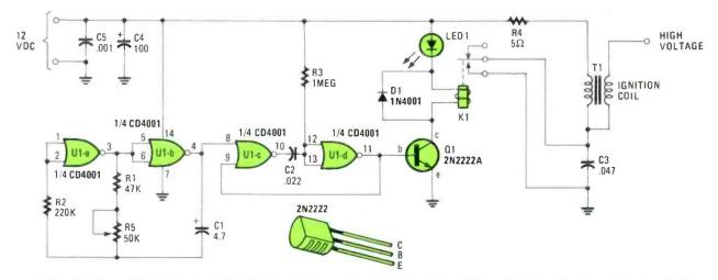
Fig. 1—The Fence Charger, for the most part, consists of a handful of easily obtainable parts. The coil, however, comes from the standard ignition system of 1960-era GMC cars. Capacitor C3 is the original component used in the system.
