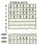
Fig. 1—This illustration of the organization of a memory chip—which is capable of storing 4K or 4096 bytes of data shows that the chip is made up of several storage locations, each having its own distinct address (0–4095).
