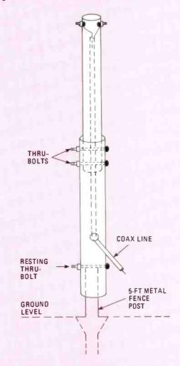
ble as needed. Connect the wires that will act as the RF pick-up element. If guys are to be used, connect them now. Use nylon stranded rope—the smallest diameter you can buy. Drop the mast over the fence post and secure with bolts. And finally, secure the guys. Taller masts can be built by using longer or additional lengths of PVC tubing.
