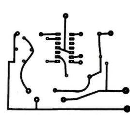
Fig. 3—Full-scale template of the display printedcircuit board for the Super ESP Tester.
