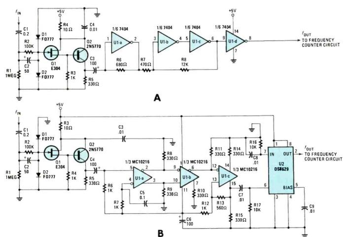
Fig. 2—Intersil's single chip frequency counters require some preconditioning before they can be expected to function properly. The circuit in A is useable at frequencies up to about 30-MHz, and may be used to directly feed a 10-MHz counter. But for higher frequencies, such as encountered in video and digital circuits, the 2 configuration is the way to go.
