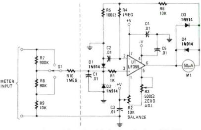
Fig. 4—This analog millivoltmeter, using the LF355 JFET op-amp, can be put together for just a few bucks. And the three-step attenuator network, consisting of R7–R9, can be expanded for greater range and versatility.
