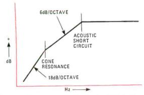
Fig. 2—The low-frequency response of an unmounted loudspeaker diminishes at about 6dB/octave in the region of acoustic short-circuit and by a further 12dB/octave below the cone resonance.
