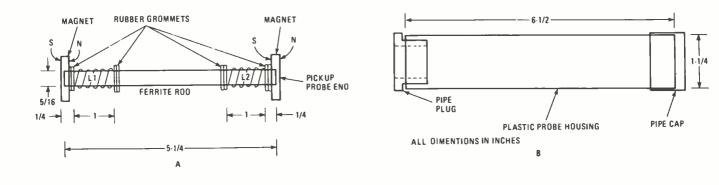
Fig. 4—The sensor probe is fabricated using the specified parts (see text for details). Grommets can be glued in place on the ferrite rod to act as a border when winding the coils.
