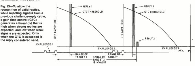
challenge I and is within radar range. Thus, the reply pulse amplitude is greater than the GTC threshold. But, REPLY 2 is invalid since it's a target's reply from challenge I and is outside the radar's range. The reply pulse amplitude, therefore, is less then the GTC threshold.
