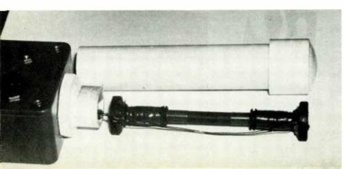
The Magnetometer's housing is outfitted with a plastic pipe plug through which the probe and the printed circuit are connected. Once connected, the probe is placed inside its PVC housing and covered with a plastic pipe cap. Then the probe assembly is affixed to the project box by pushing the PVC tubing over the plastic pipe cap.
