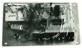
The Super ESP Tester is built on two small printed-circuit boards to allow them to be easily mounted to the back of the front panel of the project box. Note that a large electrolytic capacitor (C2) is mounted on the panel as well.
