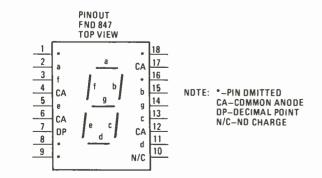
Fig. 11—A pinout-location diagram for the FND847 display module is given so that if the unit specified can not be easily obtained, substitutions may be made.
