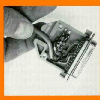
Wire the cable and switch according to Fig.,1, and carefully route the cable around the switch, so that the cable doesn't get pinched when the other hall of the hood is secured.
