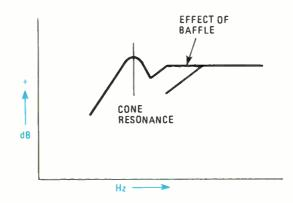
Fig. 4---Fitting a loudspeaker to a baffle pushes the 6dB/octave roll-off further down in the range. The cone resonance can become very prominent, as a result, if it's not sufficiently damped by the associated amplifier.
