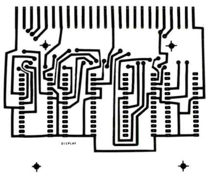
Fig. 5—The foil pattern for display board may be used as is, or modified as you see fit (see text).
