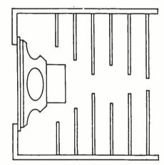
Fig.7—The "boffle" box used a succession of panels and spacers, with a circular hole in each panel, progressively smaller toward the back. The panels were designed to minimize standing waves in the box.
