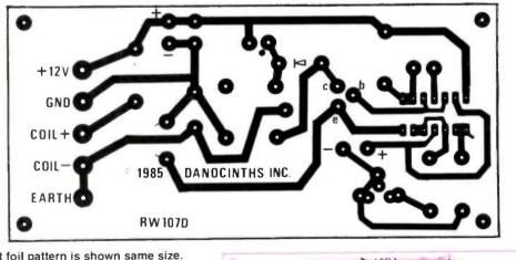
Fig. 2—Printed-circuit foil pattern is shown same size. Although, construction is not critical, using the printed-circuit board illustrated helps to cut down on errors that may damage polarized components.
