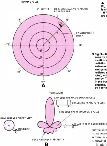
pulse (see Fig. 6). The SPI function provides a marker for the controller to identify a specific target craft from among many others, usually by making the target's blip on the PPI blink on and off.
