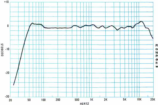
Fig.5—The frequency-response curve of a full-scale domestic loudspeaker system using Philips drivers and a Philipsdesigned, sealed enclosure. It could readly cope with low-end bass boost.
