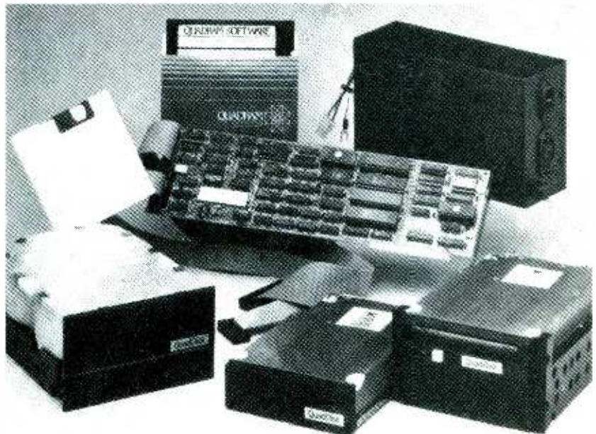
Hard disk drive units come in all shapes, sizes, and configurations. This assortment of 5-1/4 inch drives are from a single manufacturer, and are designed for use with a single computer, an IBM-compatible. There is at least one hard disk unit available for every conventional personal computer.
