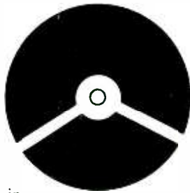
Fig. 6—Details for making an on-board power supply for use in electronic jewelry is shown. Three additional boards of the same shape and size, etched as shown are required.
