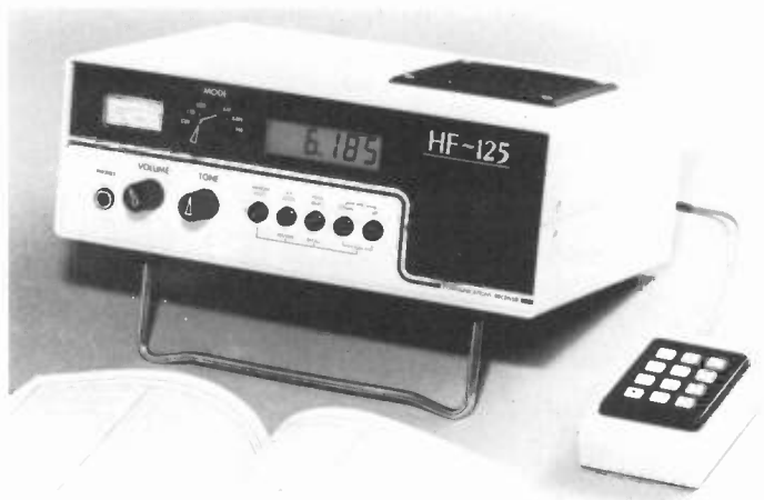
Figure 5 Behind the unassuming facade is Lowe's all-British HF-125, a high-performance synthesized set with microprocessor control. Coverage is 100 kHz to just short of 30 MHz; and among the features are 20 memories, four filter bandwidths and an exceptionally overload-resistant input stage. The keypad is optional; other extras are a matching stage for a whip antenna and a detector module giving narrow-band FM plus high-quality synchronous demodulation on AM
