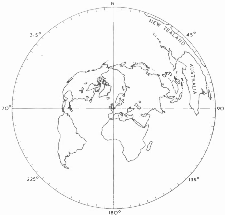
Figure 9 A great circle map, based on the UK. This is how the world appears to an amateur transmitter. Radio signals travel along great circle routes (which are the shortest routes on the globe and which on the map would be represented by straight lines radiating outwards from the centre). Such a map is essential when planning an antenna installation as it shows the directions along which signals will travel to particular countries. However, it should be noted that, in the mornings, signals to and from Australia, New Zealand and the Far East often travel the 'long way round' across South America. These directions will be exactly 180° more than those indicated on the map.
