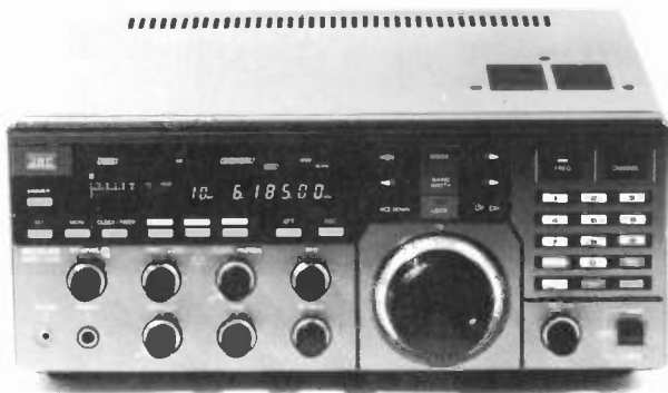
Figure 1 Japan Radio Co.'s NRD-525 receiver covers 90 kHz–34 MHz in a single band. Optional plug-in converters extend its range into the VHF/UHF region
