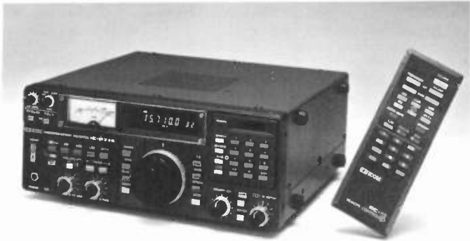
Figure 4 One of many features claimed for this Icom receiver is a virtually complete immunity to strong adjacent-channel signals. Operation can be controlled from the infra-red handset – or by a home computer
