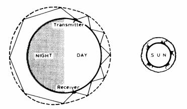
Figure 9 The change of effective height of the ionospheric reflecting layer around dusk and dawn produces the tilts that make possible chordal hop propagation for long-path transmissions, with low darkness attenuation and elimination of multiple ground-reflection losses that occur on the daylight short-path transmissions
