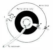
Figure 21 Coplanar twin loop (CTL) aerial. The outer, high-impedance wire loop is tuned by loading coil L and capacitance C1 which has a low value (e.g. 10pF). Damping resistance R (100 ohms variable) adjusts the Q and hence the coupling to the inner. low-impedance metal strip loop, tuned by C2 (a few hundred pF). The CTL can be adjusted to give an unidirectional null to a transmission edge-on to the loops and closest to the side carrying the loading coil.
