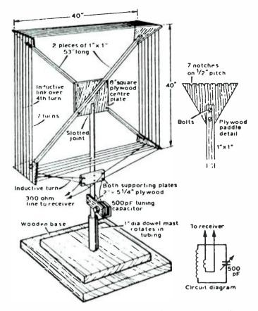
Figure 13 Constructional details of loop aerial for operation on medium waves and/or 1.8 MHz and capable of providing deep null on interfering signals
