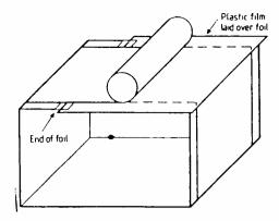
Figure 19 The box loop is made by rolling a wide strip of aluminium cooking foil round a cardboard, wooden or plastic box. Where the start and finish of the foil overlap they are prevented from shorting by inserting a sheet of plastic film. The loop can be tuned by rolling up or unrolling the foil to vary the area of overlap. The receiver is placed inside the box and coupled to it as described in the text.
