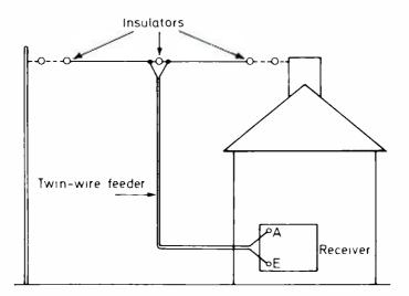
Figure 16 Simple dipole aerial
