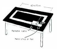
Figure 20 The horizontal loop antenna (HLA) is a wide strip of metal (sheet, aluminium foil, etc.) on an insulating support such as a table top. A gap in the loop is tuned by a variable capacitor of conventional or improvized type. The aerial is insensitive to vertically polarized signals such as local jamming but responds to long-distance ionospheric signals, which have horizontally-polarized components.
