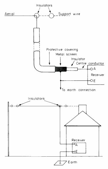
Figure 14 (a) Inverted L aerial. (b) Screened down-lead
