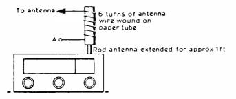
Figure 12 Using an external antenna when no socket is provided. Reception of frequencies above 15 MHz is usually enhanced by connecting point A to earth
