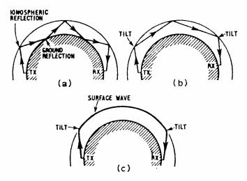
Figure 8 (a) Conventional 'HF' multihop path with two ground reflection points. (b) Chordal hop path sometimes with wave trapped between ionospheric layers. (c) Another possible form of chordal hop
