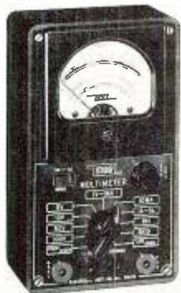
BELOW: Moderately-priced 1,000-ohms-per-volt multimeter has 31 ranges, including 0-1 volt on both AC and DC. The 3½-in. meter has a 400-microampere movement. Resistors are rated at 1% accuracy. DC accuracy rated minus 3% full scale; AC, plus or minus 5%. Electronic Instrument Co., 276 Newport Street, Brooklyn 12.
