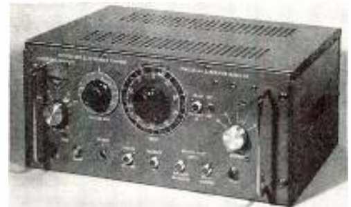
RIGHT: Time-delay generator for producing delay intervals of 10 microseconds to 10 seconds. There are 5 ranges, giving full-scale of .001 second to 10 seconds. Blocking oscillator and single-shot output wave forms are provided. Front panel is intended for 19-in. rack mounting. Rutherford Electronics Co., Culver City, Calif.
