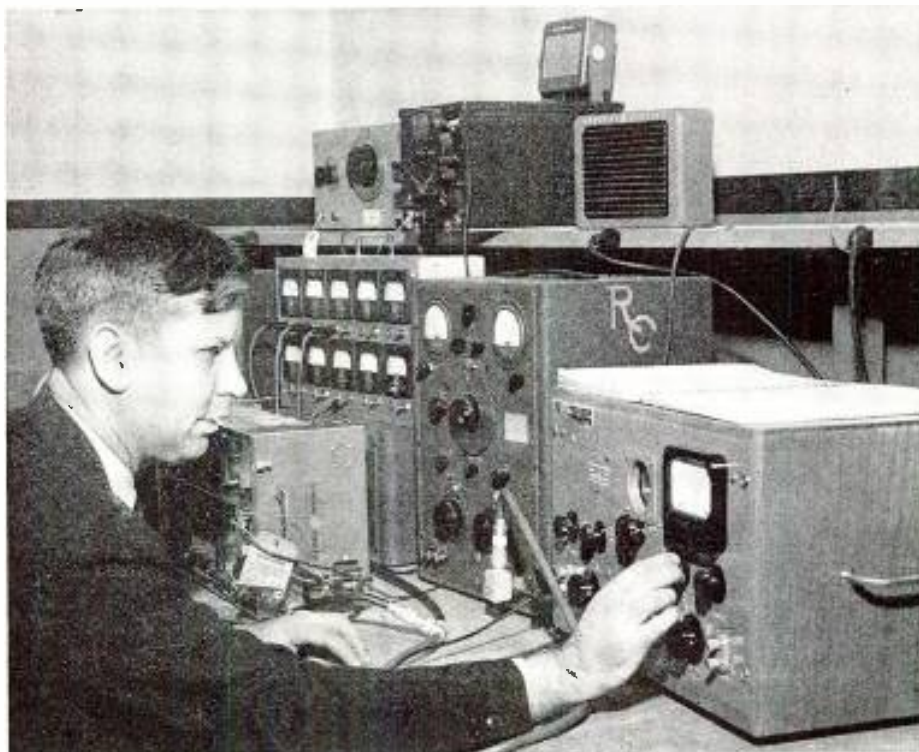
FIG. 2. SETUP FOR TESTING RECEIVER SELECTIVITY BY THE IRE 2-SIGNAL SPECIFICATIONS
