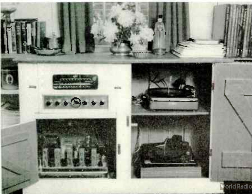
FIG. 15, RIGHT: ANOTHER WAY TO PROVIDE A CORNER MOUNTING FOR A LOUDSPEAKER. THE LOWER SHELVES OF THIS CHINA CABINET WERE REMOVED TO ACCOMMODATE THE BAFFLE. SEPARATE VOLUME CONTROL IS PROVIDED
