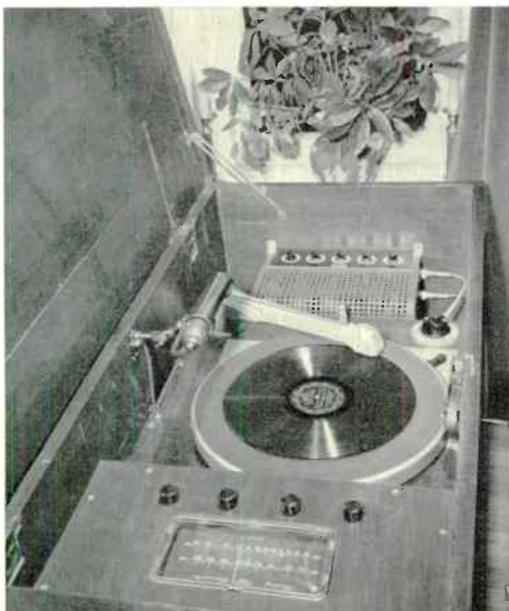
FIG. 18, LEFT: AN OLD CHEST WAS USED FOR THIS RADIO-PHONOGRAPH COMBINATION. HORIZONTAL PANELS, BUILT IN AT THREE LEVELS, HOLD THE TUNER, TURNTABLE, AND AMPLIFIER. A LIGHT ILLUMINATES THE RECORDS
