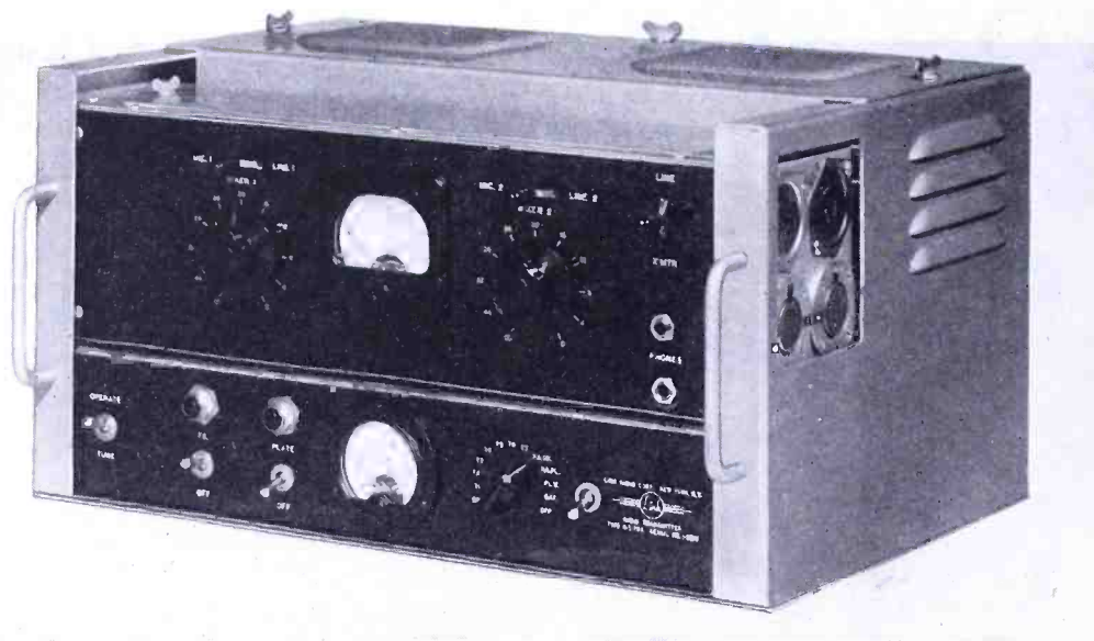
Fig. 4. Portable transmitter has pre-amplifiers, monitoring and switching circuits
