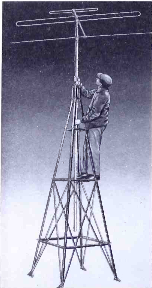
Fig. 5, left. This tower permits the mast to be slid up and down. Fig. 6, right, welded steel tower can be pushed up like a ladder. Fig. 7, above. Bevel gear is used to orient this antenna manually. Fig. 8, below. Two types of heavy 300-ohm line
