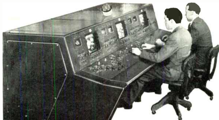
Du Mont Type TA-105-A Film Pickup Control Console. Includes saw-tooth, parabola and sine-wave shading with 5" waveform monitors for both line and frame. 12" picture monitor. Instantly accessible chassis.
