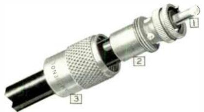
Fig. 2. Be sure that the coupling ring 3 is in place on the cable before the connector shell is soldered to the cable
