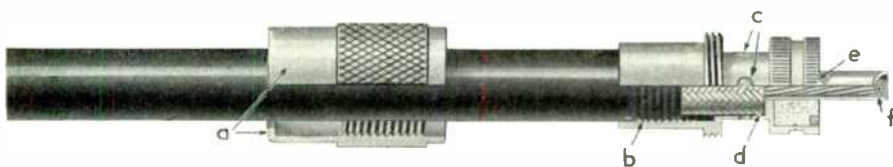
Fig. 1. Cross-section of cable and connector, with the coupling ring pushed back
