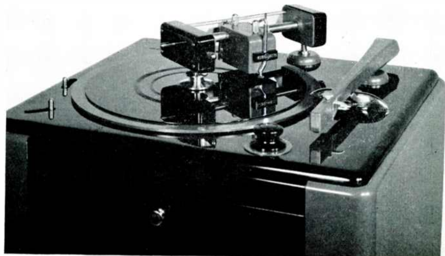
FIG. 24. A transcription turntable and recording attachment for studio operation
