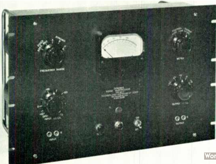
FIGS. 3 AND 4. FRONT AND REAR VIEWS OF THE DEVICE WHICH EMPLOYS DYNAMIC BANDWIDTH CONTROL TO REDUCE NEEDLESS NOISES
