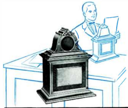
1921: The condenser microphone, designed by Bell Laboratories for sound measurement in 1916, entered the public address and broadcasting field. It provided a wide frequency range and reduced distortion.
