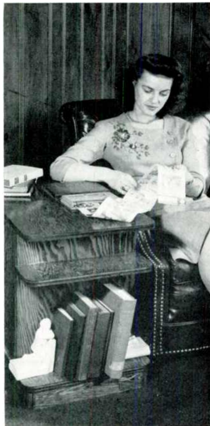
FIG. 1. FACSIMILE RECORDER BUILT INTO CONVENTIONAL CABINET
