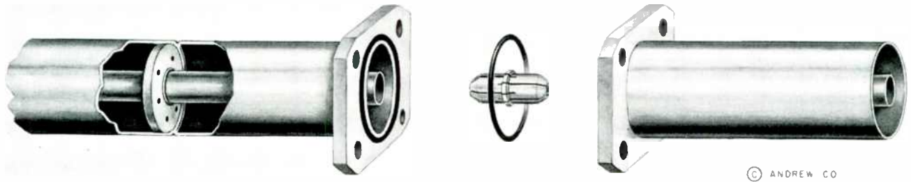
FIG. 11. CONSTRUCTION OF JOINTS FOR INNER AND OUTER CONDUCTORS, AND GAS SEAL BETWEEN 20-FT. LENGTHS
