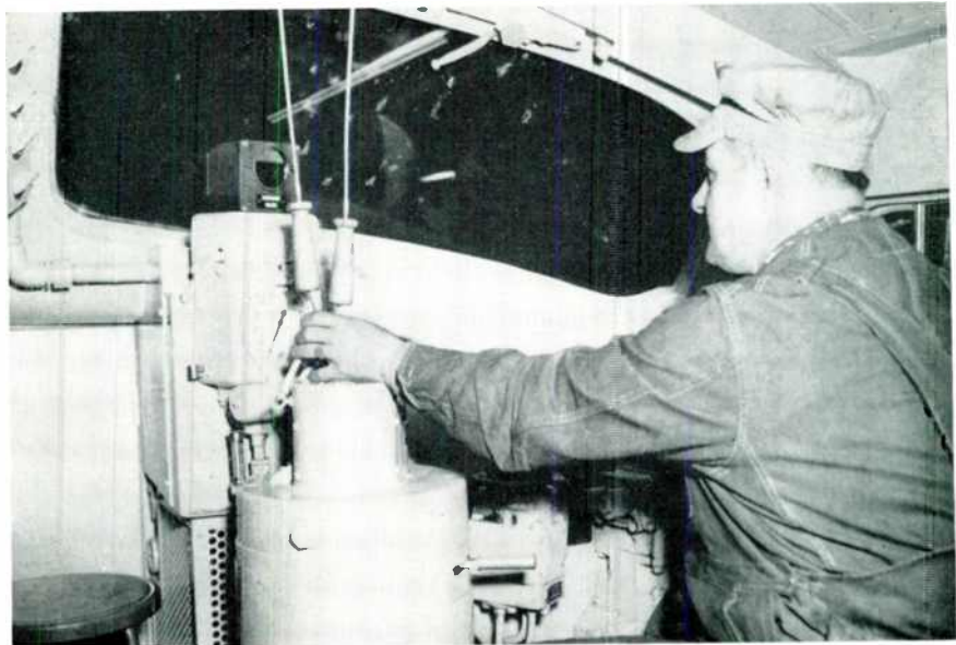
FIG. 1. RADIN DISTANCE INDICATOR IS ABOVE THE ENGINEER'S HAND
