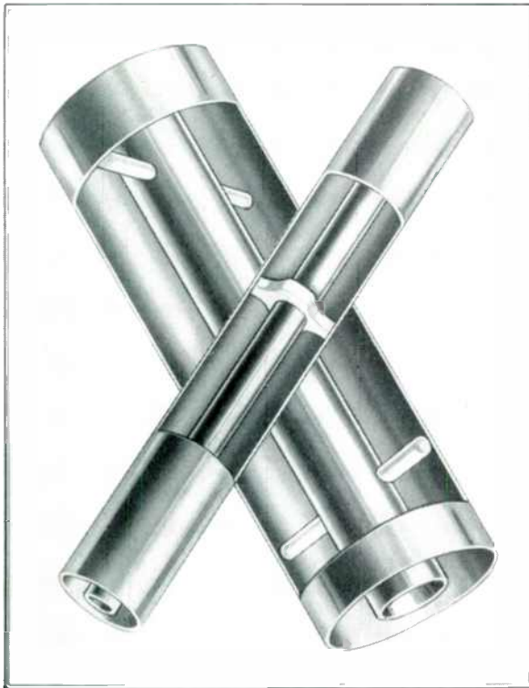
FIG. 1. INTERNAL CONSTRUCTION OF COAXIAL LINES
