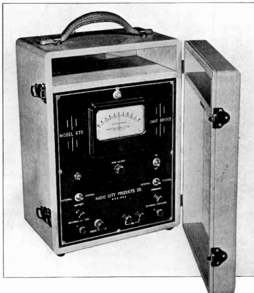
FIG. 1. THIS RESISTANCE LIMIT BRIDGE IS OPERATED BY SELF-CONTAINED BATTERIES
