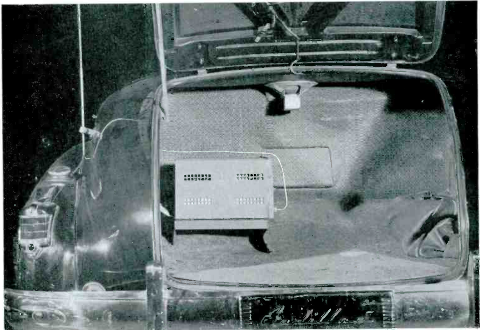
NEWS PICTURE FM Car Radio installed in Walter J. Damm's automobile is probably the first to be designed for this specific purpose. Built by REL, this receiver has a sensitivity control and signal strength indicator, shown above, calibrated in microvolts per meter. With the set crystal-controlled on W55M, Walter Damm can check the Milwaukee Journal's FM station, of which he is general manager, by the direct-reading meter. Speaker, mounted at the top of the luggage compartment, talks into the car
