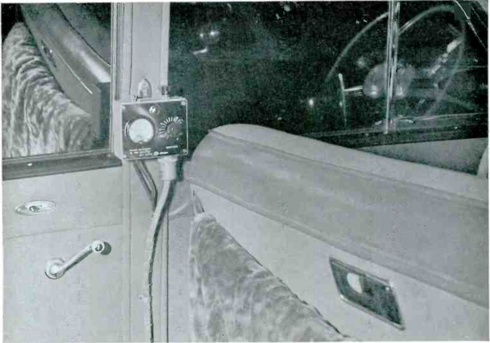
NEWS PICTURE FM Car Radio installed in Walter J. Damm's automobile is probably the first to be designed for this specific purpose. Built by REL, this receiver has a sensitivity control and signal strength indicator, shown above, calibrated in microvolts per meter. With the set crystal-controlled on W55M, Walter Damm can check the Milwaukee Journal's FM station, of which he is general manager, by the direct-reading meter. Speaker, mounted at the top of the luggage compartment, talks into the car
