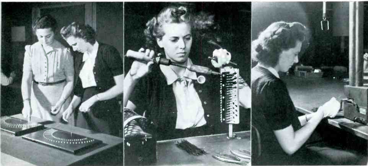
MISS DOROTHY MITCHELL TESTS GERALDINE'S SKILL AT WINDING WIRE OVER PINS. THEN, AFTER LEARNING HOW TO BURN INSULATION FROM WIRES, SHE TACKLES THE JOB OF SOLDERING WIRES TO TERMINAL BLOCKS. USUALLY, SIX BLOCKS ARE WIRED BEFORE ADEQUATE SKILL IS ATTAINED
