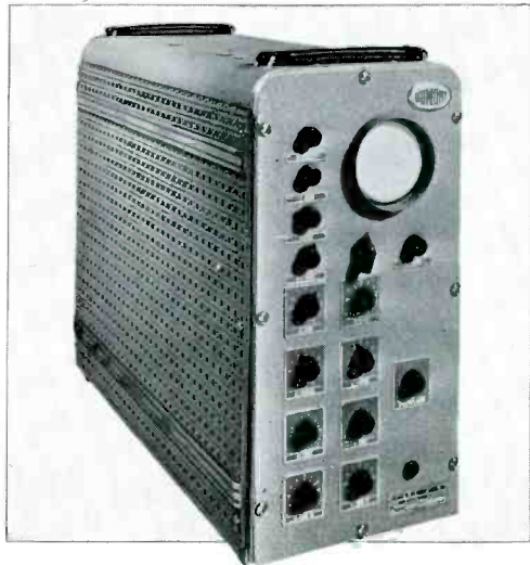
FIG. 5. TYPICAL CONSTRUCTION OF PORTABLE CAMERA CHAIN UNITS. THIS INSTRUMENT IS A SHADING GENERATOR
