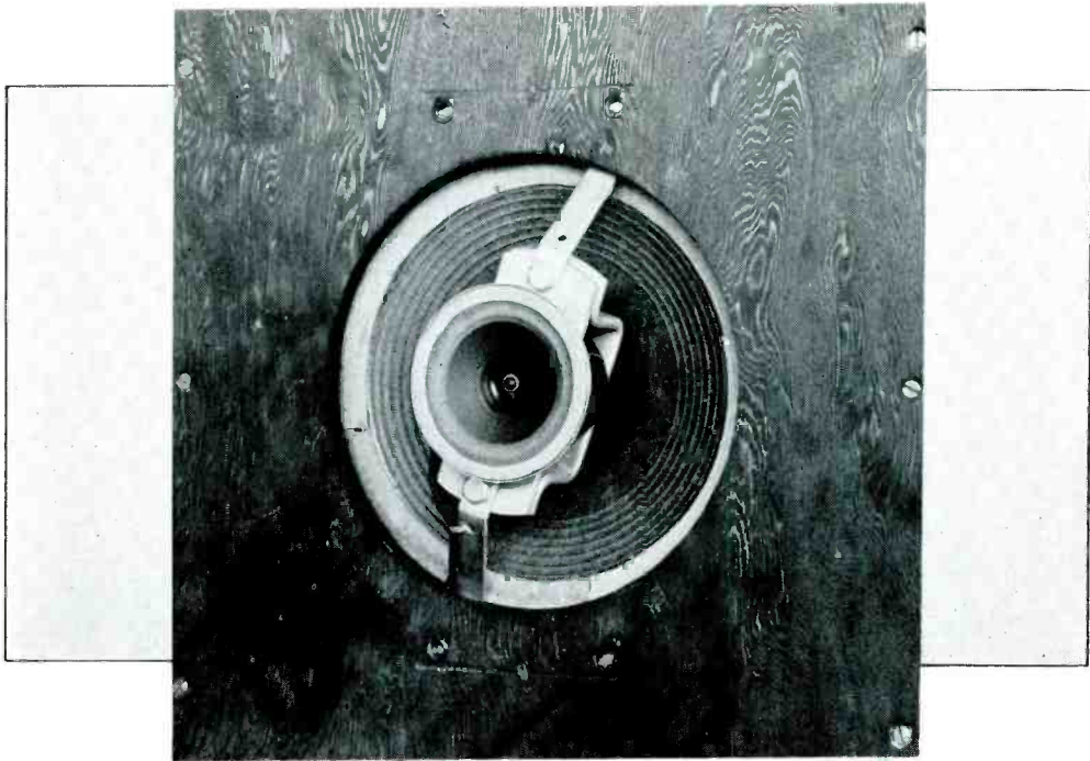
FIG. 2. THE STROMBERG-CARLSON CONCENTRIC SPEAKER MOUNTED ON A BAFFLE BOARD
