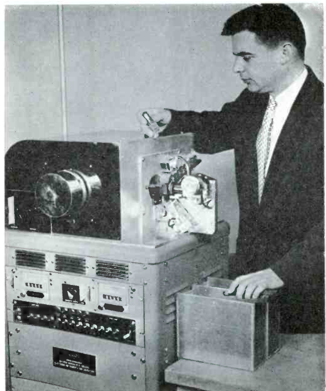
FIG. 9. BELOW: THIS MACHINE BONDS UP TO 4 CAPACITORS ON A WAFER FIG. 11, RIGHT: PART OF THE MODULE ASSEMBLY SECTION OF MPE PLANT
