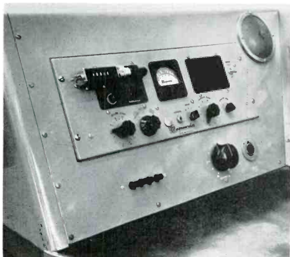
FIG. 8. CONTROL PANEL FOR ONE TAPE RECORDER. NOTE COUNTER AT LEFT OF METER. FIG. 9. TOP PANEL OPENS FOR LOADING NAB-SIZE TAPE REELS
