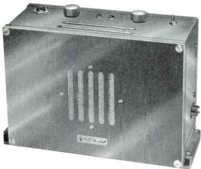
FIG. 2. CASE CONTAINS CONTROLS, TRANSCIEVER, POWER SUPPLY, SPEAKER
