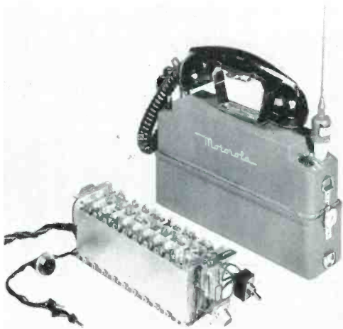
FIG. 9. VIEW OF A HANDIE-TALKIE AND A 3-UNIT CHASSIS FITTING IN THE UPPER COMPARTMENT
