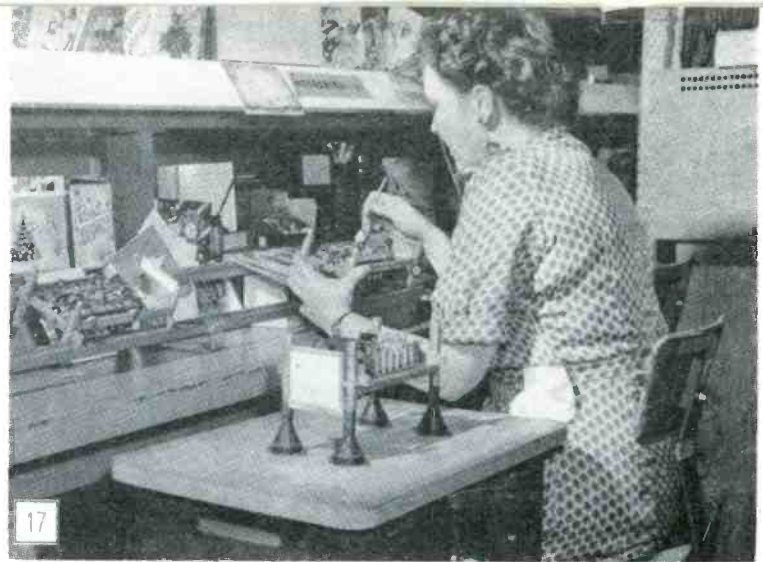
FIG. 17. AT END OF ASSEMBLY LINE, EACH CHASSIS IS RUN ON SHAKE-TABLE
