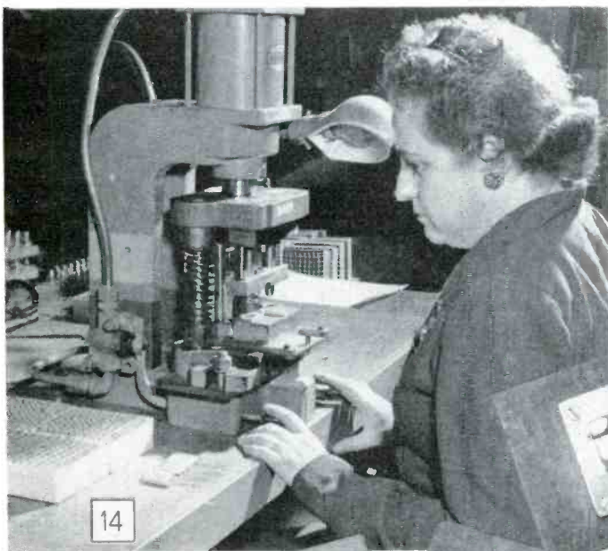
FIG. 12. SOLDERING GROUND WIRES FROM THE TUBE SOCKETS TO THE CHASSIS FIG. 14. LEADS FROM THE SUBMINIATURE TUBES ARE LAID IN A SLOTTED FIXTURE, AND ARE CUT TO LENGTH IN THIS PNEUMATIC PRESS
