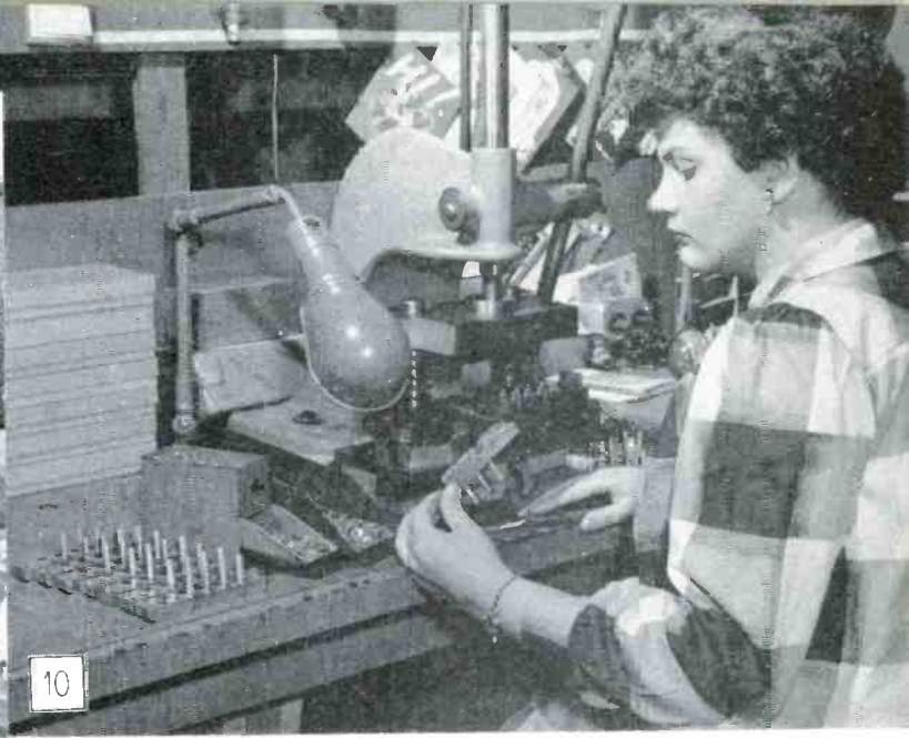
FIG. 9. POWER-DRIVEN THREAD GAUGE IS USED TO INSPECT EACH OF 36 THREADED HOLES. FIG. 10. SOCKETS ARE PRESSED INTO STEEL CHASSIS, ON WHICH TUBULAR CONDENSERS ARE ALREADY SOLDERED. FIG. 13. ASSEMBLY COMPRISES A DIE-CAST ALUMINUM CHASSIS, AND TWO CHASSIS FORMED OF SHEET STEEL
