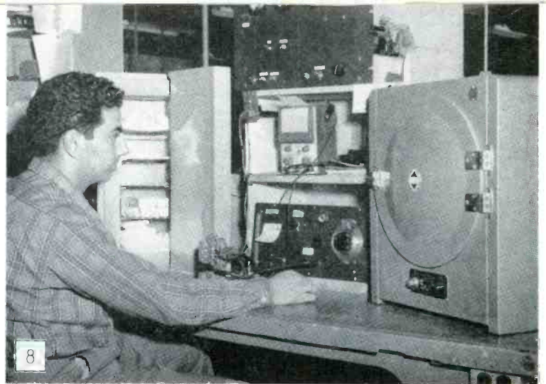
FIG. 8. CHECKING DRIFT AFTER HEATING IN OVEN, RIGHT, AND COOLING IN DRY ICE CHAMBER
