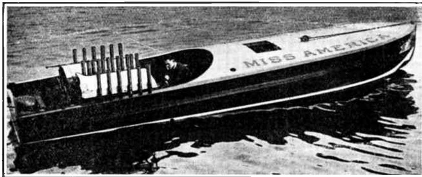
Miss America has two Liberty engines to give it record breaking speed
