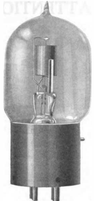
The Moorhead VT Amplifier-Oscillator
