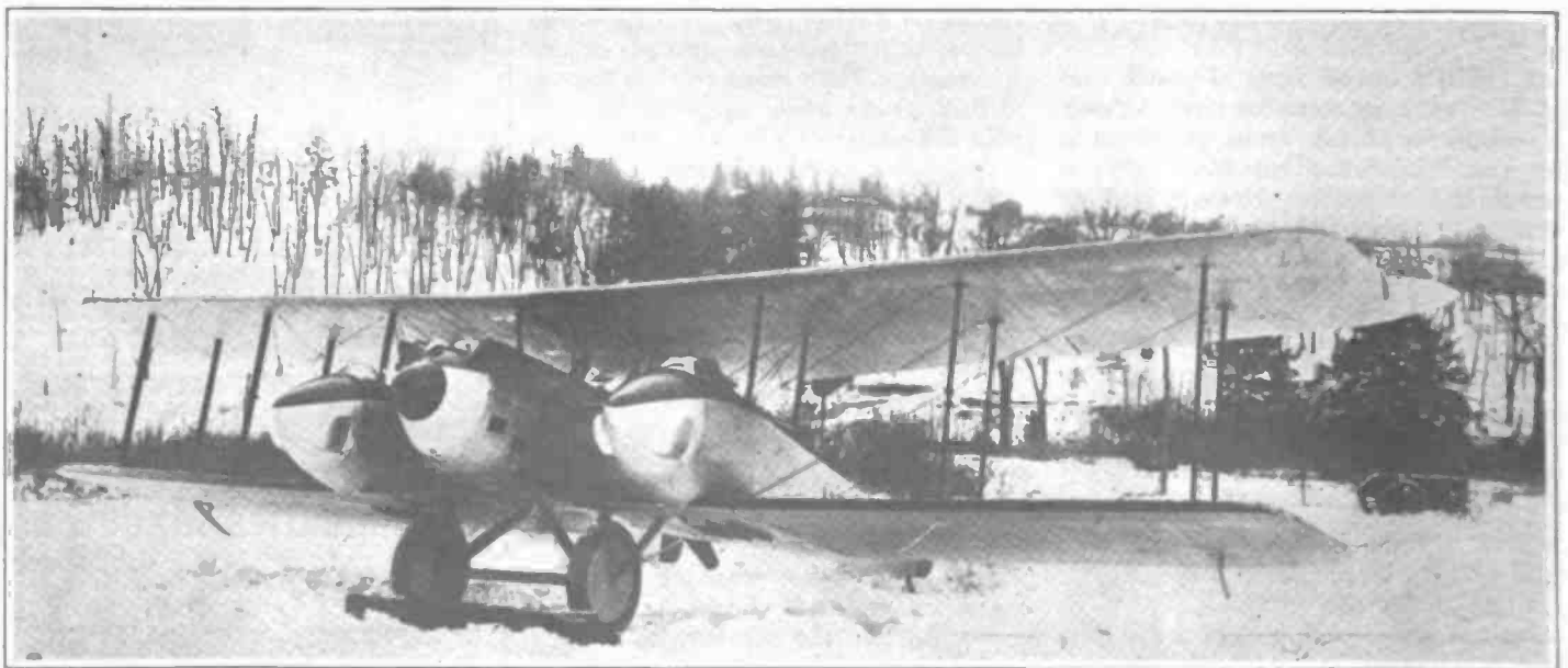
Three-quarter front view of Thomas-Morse mail plane showing central nacelle for engines and twin fuselages for pilots and mail
