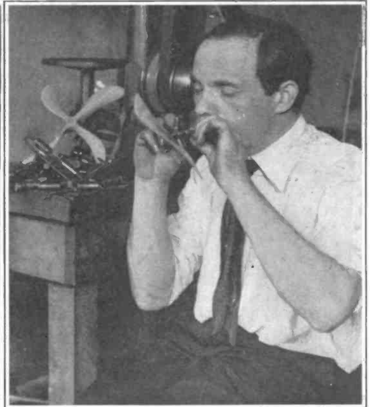
A sensitive drill press can be used to "run in" a compressed air motor. At the right one method of testing for free running is shown
