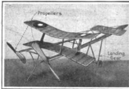
Fig. 2. Rear view of the R.O.G. biplane flier
