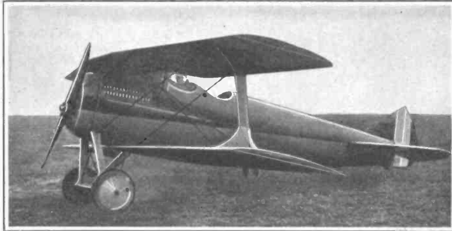
Improved Spad Biplane capable of a speed of 187 miles per hour, uses 300 horsepower Hispano-Suiza engine
