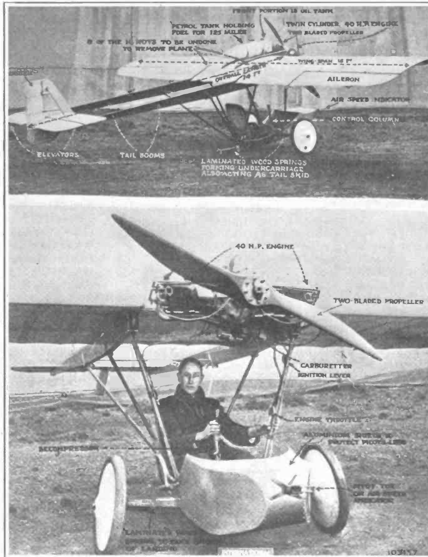
A light weight monoplane that the enthusiastic designer calls "the motorcycle of the air"
