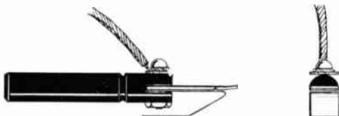
Fig. 8. Pressing the spring opens the clip to take the wire.
