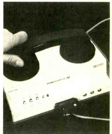
Using the modem is simple. You simply dial up the computer, wait until you hear a tone in the handset receiver and then force the handset into the muffs. Make certain the handset is firmly seated in the muffs to keep out any extraneous room noises.
