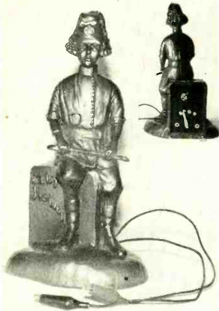
The "Baby Jacquelin" crystal radio statue is of unknown origin. The insulated alligator clips are a recent addition.
