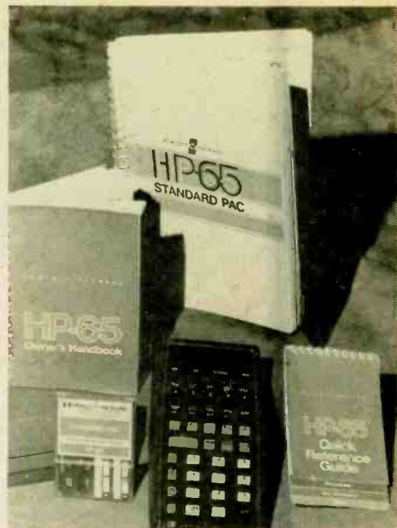
The HP-65 and its supporting software. Packaged with the calculator are user aids such as reference booklets, instruction manual, pre-written programs—and a selection of pre-recorded, magnetic card programs.
