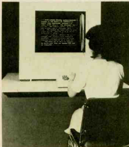
The world's largest liquid crystal display system is shown in operation at the offices of Hitachi, Ltd., one of the three Japanese-based companies who have been engaged since 1972 in a joint research project to develop a large-area liquid crystal display.
