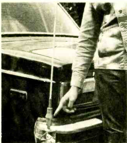
One of the best bumper-mounted antennas, with a springy base-loading coil. 108-in. whips tested out best.
