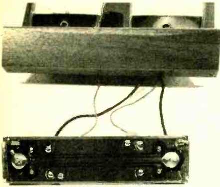
Middle foil of printed circuit is the center conductor; on either side of it are the forward and reverse power sensors.
