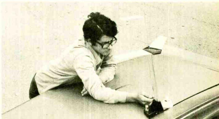
Here noble assistant tightens mast holding "wing" antenna with a coin. When car is parked take the wing with you, or it's likely to fly away from your car fast!
