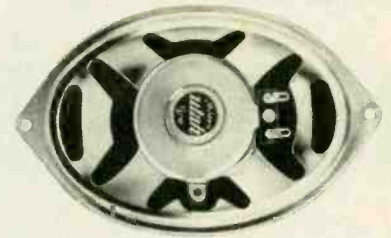
Fig. 9. Speaker terminals are on little insulated terminal board on the speaker frame.
