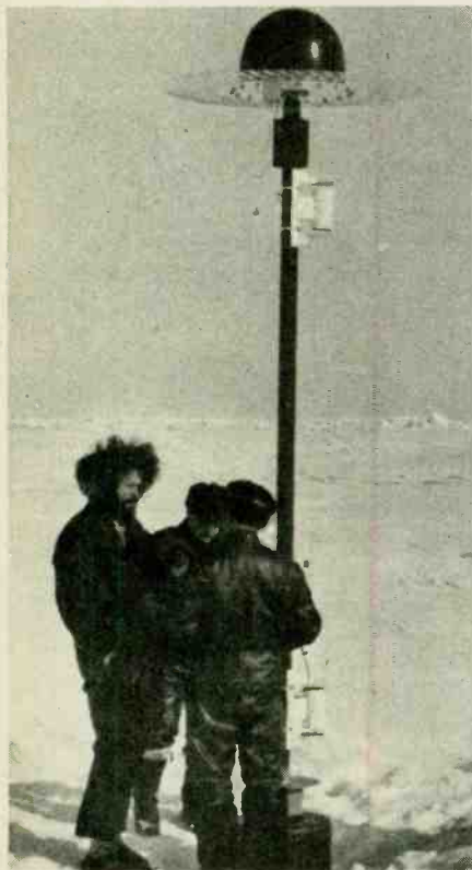
The Vibrasense pressure-sensing device atop this data buoy is used in calculating wind stresses and other climatic conditions.
