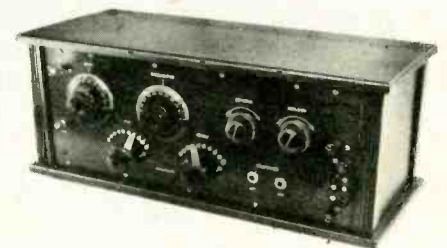
Fig. 1. Before kits really became popular, radio buffs built their own from scratch. This 2-tube regen is typical of the period.
