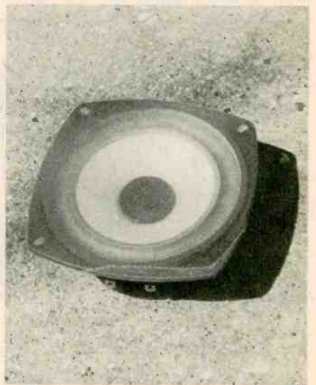
Fig. 5. If you cut and wrap the pantyhose carefully it should look like a factory installation.
