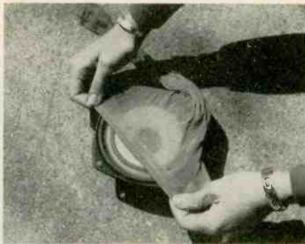
Fig. 4. Just one speck of dust in the cone from installation will rattle for ever and ever. But if you wrap the speaker in an old pantyhose (or even new pantyhose of the 2-for-a-$1 variety) you'll be able to keep chips out during installation, and the heavier dust—which also rattles—that settles in after the speakers are installed. Leave enough slack in the material so it can be completely wrapped around the speaker when you're finished.
