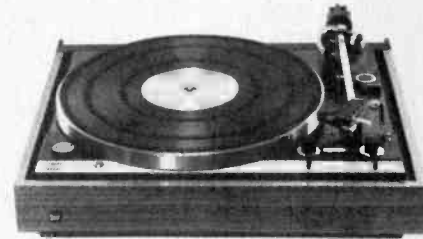
Dual's 701 has a direct-drive motor, which is an all-electronic low-speed brushless DC type with Hall-effect feedback control. There is separate anti-skating for conical and elliptical styli, an 8% pitch-control for each speed, and a built-in illuminated strobe; $350.00.
