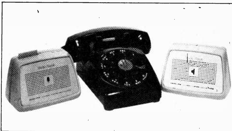
A standard size desk telephone gives a good idea of the conference phone's scale. In actual use there's no need for the conference phone to be near the regular telephone as the call can be answered directly at the conference set. The receiver has a combination power/line on-off switch and a receive volume control on top of the cabinet. The switch is push-for-on/push-for-off.
