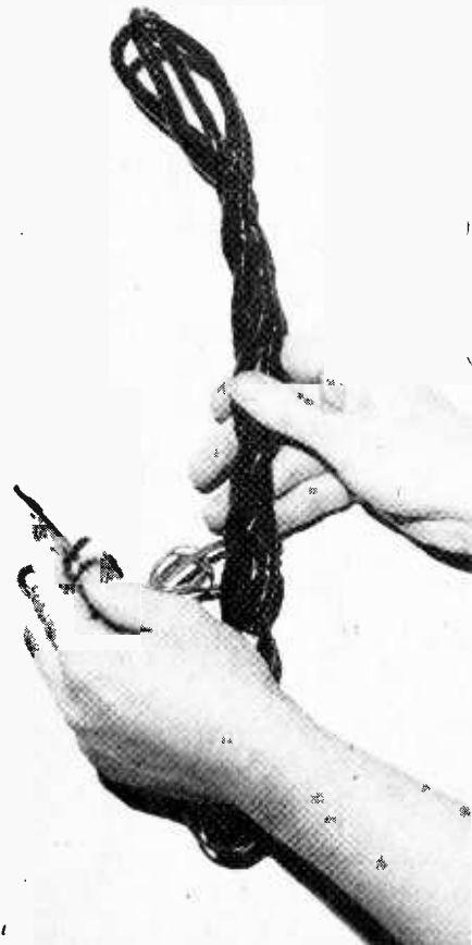
Degaussing coil for automatically demagnetizing larger color cathode ray tubes is part of the NRI 25-in. TV kit and your training.
