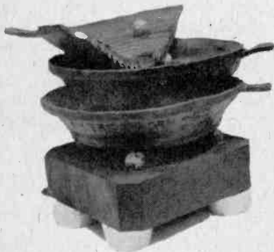
1. This is a battery made in Switzerland in 1904. The pans are treated on one side with a negative substance and on the other with a positive substance. The balls between the pans are insulators. Only a few of these batteries were ever produced, since the company that made them went out of business in 1905. This particular battery is believed to be the only one of its type still in existence.
