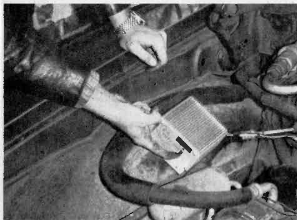
Fig. 6. Flip the switch on the Tiger 500 to CD and you can select either CD operation or normal Detroit ignition operation.
