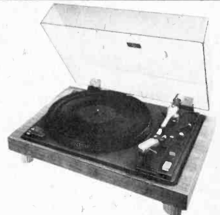
From Kenwood, the direct-drive KP-5022 features an 8-pole, brushless DC servomotor directly coupled to the center of a massive, 12-inch solid die-cast aluminum alloy turntable that has an engraved stroboscope pattern around its rim. A pilot lamp is provided for overhang adjustment; $299.95.
