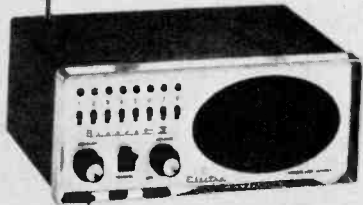
4 bands, 8 channels: Electra Bearcat IV. $179.95 for 30 to 50, 150 to 174, 450 to 470, and 470 to 512 MHz.
