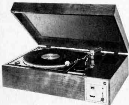
Toshiba's SR-50 uses a photoelectric pickup whose stylus modulates a beam of light, resulting in a moving mass of only 0.3 milligrams. The preamp in the base contains an electronic optimum stylus-force and anti-skating gauge. End-of-record sensing is also photoelectric; $449.95.
