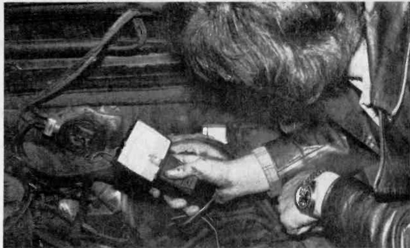
Fig. 7. CD ignition might raise the motor idle speed so use a tach to check it out. If the idle rpm is high just pull it down to specs with the carburetor's idle speed adjustment screw.
