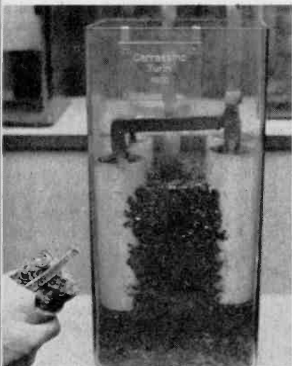
2. This is an "accumulator" made by Carassino of Turin, Italy, in 1900.
