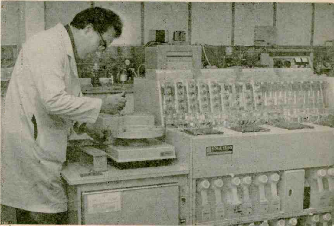
The SMA 12/60 (above) can perform twelve different chemical analyses at the rate of sixty per hour. A technician is pouring a new blood-plasma sample into the machine.
