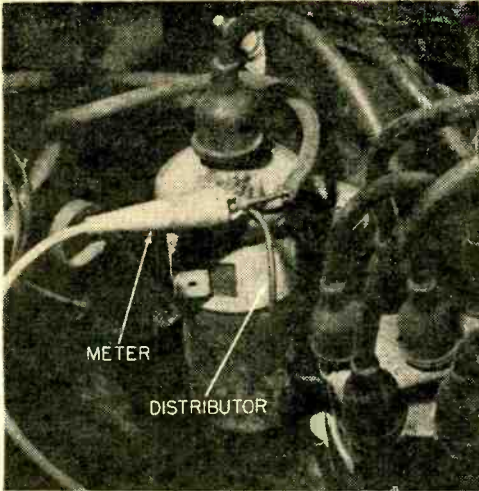
Clip "meter" wire from dwell/tach to ignition coil minus terminal. Look for "distributor" wire. It runs from the (-) terminal to the base of your distributor.
