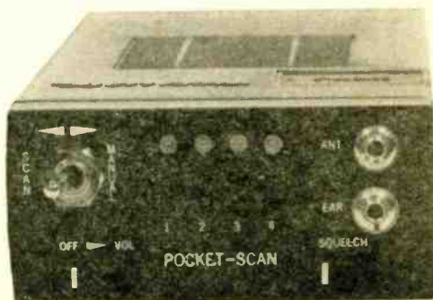
All controls are mounted on top including individual lock-out for each VHF channel.
