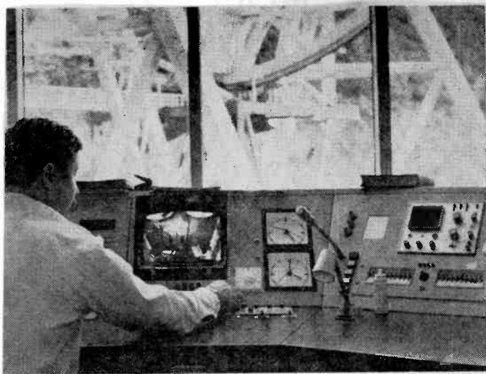
From the control building (left) the scientist sitting at the control console relies on television to see the entire structure. The precise time is important, too! Scientist (right) peeps into scope while adjusting local clocks to an atomic standard.
