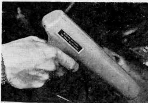
Heathkit's Inductive Pickup Light is powered by the car battery. Pickup can be attached to spark plug lead even with engine running.
