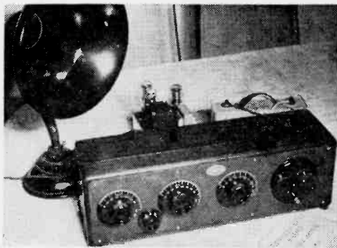
Carefully install the receiver chassis and front panel into the cabinet (left) Photo at right shows the completed Atwater Kent in restored condition and ready to play. Note B+ power supply and filament battery behind unit.
