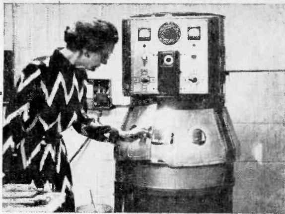
FadeOmeter test at U.S. Testing Co. creates simulated sunlight to test fabrics for fading. Here, draperies reveal sunfastness.
