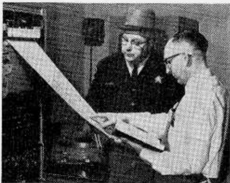
Sheriff O. B. Weatherstroom watches while senior chemist William S. Best compares recorded measurements from the GE X-ray diffraction equipment with known measurements in the book distributed by the American Society for Testing Materials.
