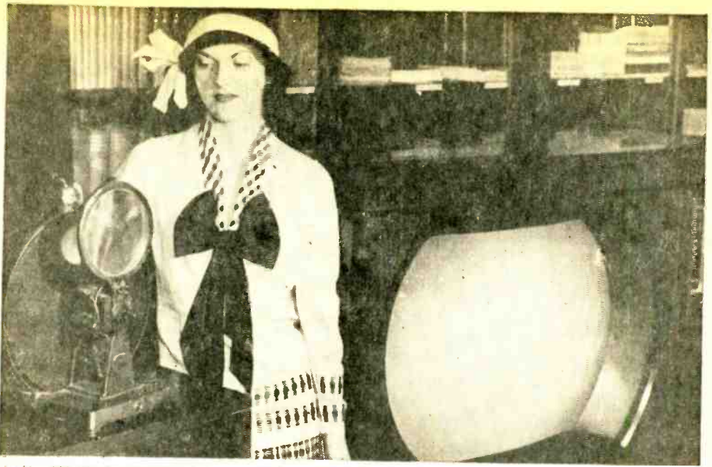
Jenkins 102 "Radiovisor" of 1929 contrasted with 1952 DuMont Royal Sovereign. DuMont had 30-in. screen.
