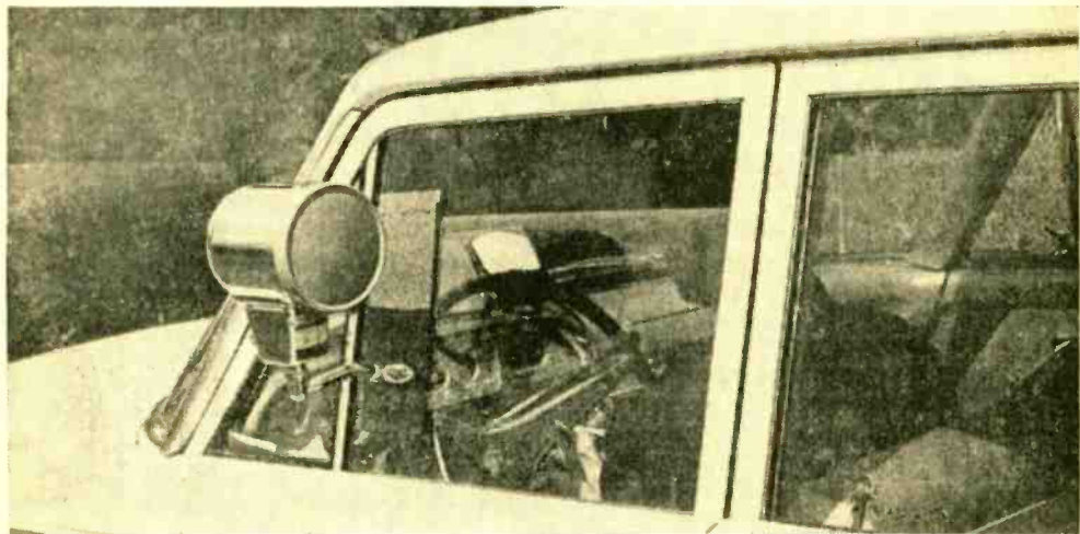
Three devices used by police in radar-trap setups: above, radar speed meter installed in glove compartment with automatic chart recorder at right (entire installation would be unnoticed by passing motorist); right, portable radar unit; below, radar antenna on window.
