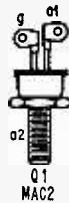
Two semiconductor devices, a Triac (Q1) and a bilateral trigger diode (D1), control current over each half-cycle of AC. Note outline of Triac.
