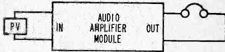
Fig. 18. Want to listen to a light beam? It's easier than you think. Simple diagram proves the point.
