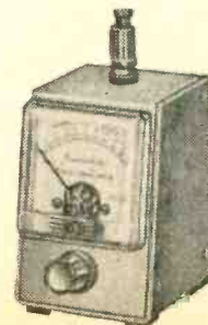
Measure relative transmitter power of Ham, marine, commercial or CB rigs with this small Heathkit PM-2.
