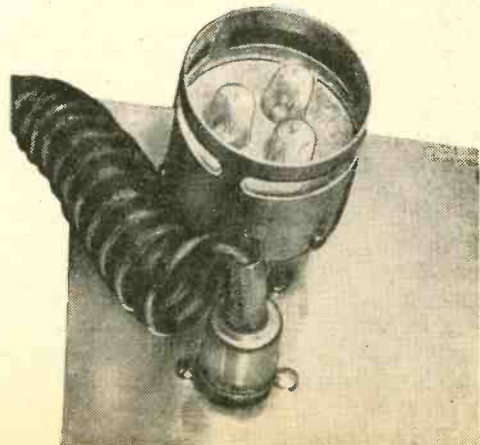
Fig. 15. Dummy load for low-power transmitter uses three pilot lamps. Current flow changes resistance.
