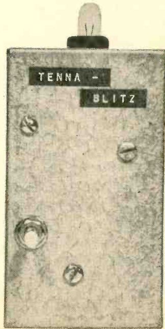
All wired up and ready to go, completed unit has but one control—switch S1, whose shaft extends from lower left of front panel. Flasher lamp I1 appears at top of chassis box; its base is pressed into 1/2-in. rubber grommet.
