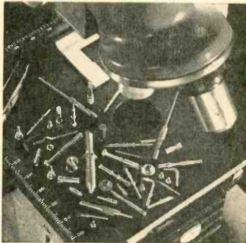
You can tell how small small is by comparing machined parts to centimeter scale on microscope stage platform.
