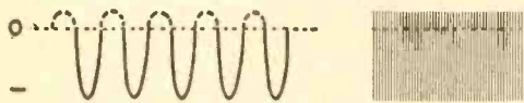
Fig. 2. Non-linear amplifier results in signal-stripping waveform shown. Average voltage below line must be subtracted from average voltage above zero line. The resulting signal distortion is indicated in Fig. 9.
