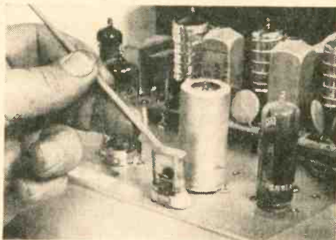
Many sideband rigs employ fixed crystal oscillator for heterodyning signal to desired frequency (rod points to crystal associated with mixer in this unit).
