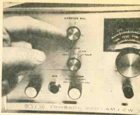
Typical SSB rig (this is an EICO Ham transmitter) incorporates Mode switch to enable operator to select CW, AM, or SSB operation at will. Finger points to knob labeled "Carrier Bal" which serves as fine-tuning adjustment of modulator stage to eliminate RF carrier.
