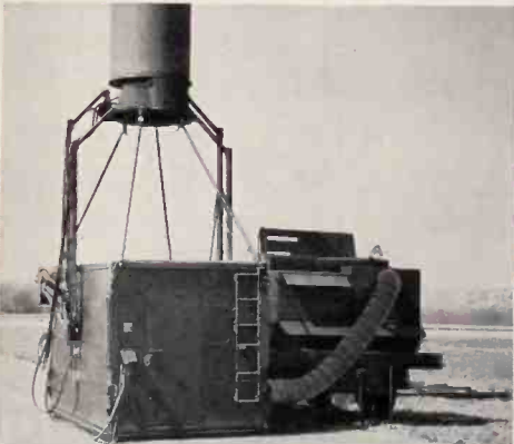
Radio Set AN/TRN-6 The TACAN Ground Station — Transportable by plane or truck. Shelter dimensions: 11' 8" long, 7' high, 6' 5" wide.
