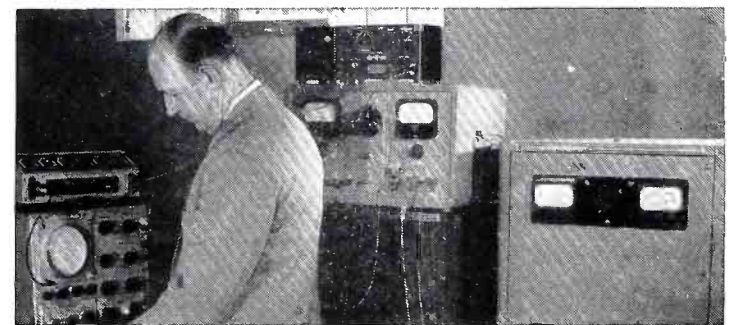
Testing pulse transformers. This set-up can simulate the operating conditions of pulse transformers up to one million volts.
