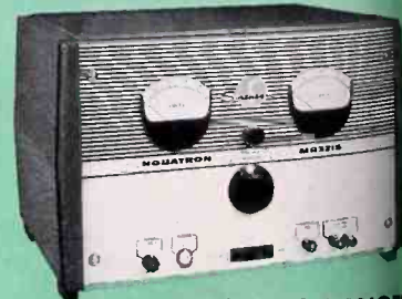
Model MR3215 MAGNETIC RANGE (tubeless wide-range variable regulated DC source).
