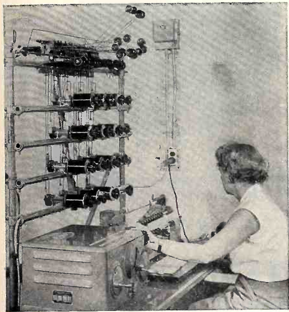
SEMI-AUTOMATIC WINDING MACHINE (PROTOTYPE WORK). The Prototype and Sample Department covers approximately 2,500 square feet and is completely equipped to perform all operations from winding to finishing independently of the Production Department.
