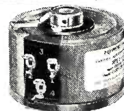
TYPE 10-1002 INPUT: 120 volts, 50/60 cycle, 1 phase. OUTPUT: 0-120 volt, 1.25 amperes, .15 KVA. Complete Rotation.
