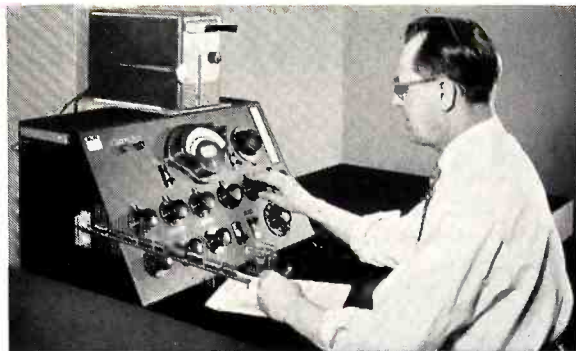
Allen-Bradley engineer checking resistors after humidity test.
