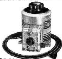
TYPE 116 INPUT: 120 volts, 50/60 cycle, 1 phase. OUTPUT: 0-140 volts, 7.5 amperes, 1 KVA. Enclosed with Cord-Plug, Receptacle, Fuse, Switch.
