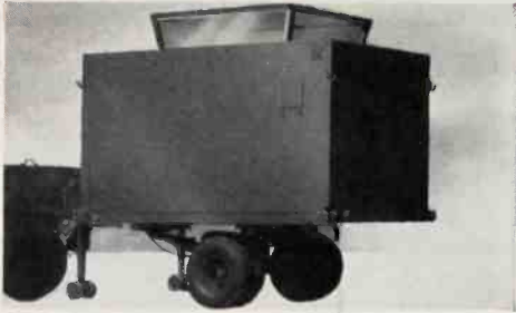
Air Traffic Control Central — Mobile, self-contained, fully equipped for control tower operations. Powered by mobile generators or commercial power. Transportable by air, land or sea.
