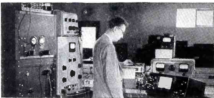
The measurement of filter characteristics as an aid in the design of the most efficient and economical filters.
