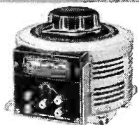
TYPE 136 INPUT: 120 volts, 50/60 cycle, 1 phase. OUTPUT: 0-120/140 volts, 20.0 amperes, 2.8 KVA. Exposed Terminal Connections.
