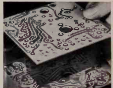
G-E "Thru-Con" Printed Circuit Boards offer positive connection through the holes, without staking pins, patterns on both sides if needed. Printed circuitry cuts assembly time; eliminates product bulk, weight; reduces inspection time, parts inventory.
