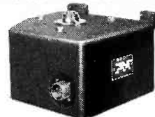
TYPE 1126-1001 INPUT: 115 volts, 400/800 cycle, 1 phase. OUTPUT: 0-130 volts, 15 amperes, 1.95 KVA. With a Dust-Proof Container.
