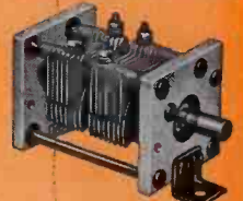
"VU" Permits use of "lumped constant" circuits up to 500 MC. Two sections in series eliminate rotor wiper. Pyrex glass ball bearings eliminate noise from usual metal-to-metal bearings.
