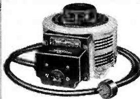
TYPE 2PF136 INPUT: 120 volts, 50/60 cycle, 1 phase. OUTPUT: 0-120/140 volts, 20.0 amperes, 2.8 KVA. With Cord-Plug, Fuse, Receptacle.
