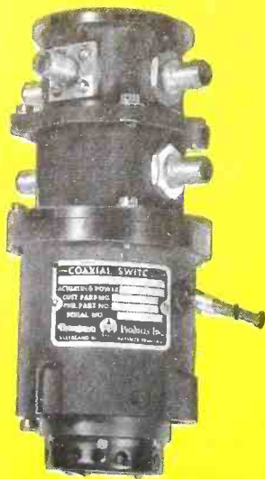
Model CA-31, 2P2T Sensing or Lobing Switch, 115 volt, 380-1000 cycle AC motor actuator. Switching speed, 15-35 Rev./sec. For use with RG-58/U cable.
