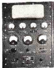
RF Power Output Test Set for Vacuum Tubes
