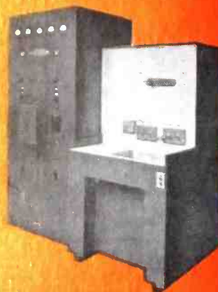
Standard 40 KW High Frequency Induction Heater with Worktable and Quenching Facilities for Special Application.
