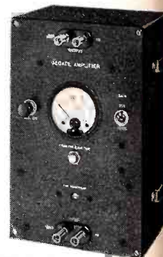
MODEL 220 A BATTERY OPERATED DECADE AMPLIFIER gives exact voltage gains of 10 or 100, permitting a corresponding increase in voltmeter sensitivity from 10 to 150,000 cycles.
