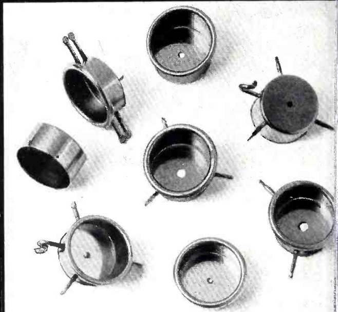
NO. 2 GRIDS and PINNING NO. 2 GRID ASSEMBLIES
