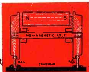
Diagram shows how magnetizing force is supplied by external stationary Crucible permanent magnet and non-magnetic axle. Wheels are sintered steel.
