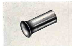
Seamless nickel tube, Flared both ends. .200" I.D. x .005" Wall x .527" long. Print #ET19-1.
