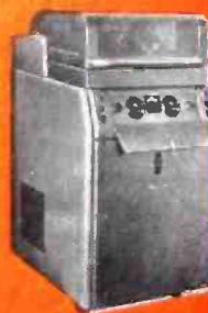
10 KW Preform Dielectric Heating unit with two timers.
