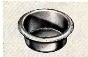
No. 2 Grid Cup, 305 Stainless Steel, Rolled edge. .499" O.D. x .010" Wall x .262" long. Print #EP37-1.
