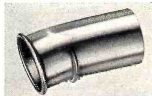
Weldrawn, 305 Stainless Steel, Rolled and bent 10°. .499" I.D. x .010" Wall x 1.050" long. Print #ET47-2.
