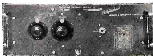
Type 706 BROADBAND MICROWAVE OSCILLATOR 3.6—7.3 kmc
