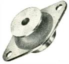
These units utilize the properties of rubber in halanced compression and shear. They provide large deflection ratings together with high load capacity, small size, and exceptional stability. Have equal spring rates in all directions – mount at any angle – absorb vibrations for every plane. Unit loadrange 50 lbs. to 2500 lbs. Write for the Isomode Design Chart.
