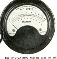
The INDICATING METER used on all BALLANTINE VOLTMETERS features a single logarithmic voltage scale and uniform decibel scale. Makes readings especially easy. Accuracy of indication is 2% at any point on the scale.
