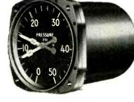
TELETORQUE UNITS -precision built selsyn type units for remote indication. Accurate to ±1 degree. Actuated by units producing as little as 4 gr/cm of torque.
