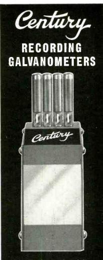
For photographic recording of d.c. or a.c. currents with "flat" frequency response to as high as 2500 cycles per second. Available in a wide range of natural frequencies, all having high factors of sensitivity and dynamic balance. Their tubular hermetically sealed construction insures long-lived dependability and ruggedness. Magnetic assemblies are constructed for 2, 4, 8, 12 and 14 element mounting.
