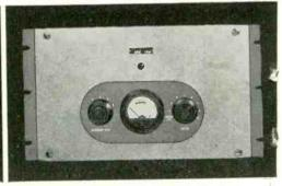
41-A PEAK LIMITING AMPLIFIER controls program peaks, removes cause of overcutting and distortion in recording and overmodulation in broadcasting. Serves simultaneously as a line amplifier; its 60 db gain adequately compensates for line losses due to pads, equalizers, etc. Vertically mounted chassis, all circuits accessible. Meter and selector switch indicate amount of limiting and current readings of all tubes.
