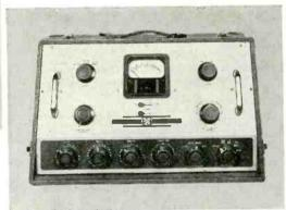
THE 90-B PORTABLE RECORDING AMPLIFIER unit incorporates the following: three channel mixing pre-amp. and line input — response: NAB, 78 rpm, and flat (30-15,000 cps)—high and low frequency equalizers—outputs for one or two turntables or a line. Provision for automatic equalization.
