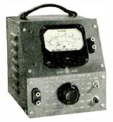
—hp— 400C Vacuum Tube Voltmeter
