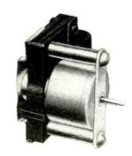
Medium-duty motor, type B Torque rating of various models from .015 pound-inch at 60 rpm to .375 pound-inch at ½ or 1 rpm at 60 cycles 115 volts.
