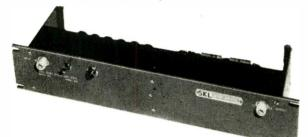
A two-stage traveling wave amplifier in which reflections are reduced to a minimum because degree of coupling between coil sections has been carefully chosen, and terminating sections of delay-lines can be varied. This permits adjustment of response characteristic to fit particular appli-
