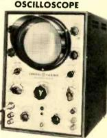
TYPE ST-2A - A new, general purpose oscilloscope. Wide frequency response-from DC to 500 kc, and with gradually reducing response to higher frequencies. High sensitivity. Sturdy construction. Voltage calibrator, Z-axis input, and DC input coupling to both amplifiers.
