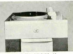
64-A TRANSCRIPTION TURNTABLE, with many exclusive features, is directly gear driven at both  $33\frac{1}{3}$  and 78 rpm, using a separate motor for each speed. Completely eliminates error in total speed regulation, reduces mechanical disturbances to a new minimum. Double throw mercury switch changes speeds. At  $33\frac{1}{3}$  rpm full turntable speed is reached within about  $\frac{1}{8}$ revolution.
