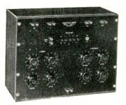
IMPEDANCE RANGE: One millibeary to hearies in five ranges, inductance values read directly from a four dial decade multiplier switch. This range can be extende 10,000 hearies by the use of an external scheme.
