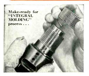
The coiled resistance element is threaded on the molded core
