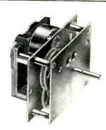
Heavy-duty motors, C types Torque ratings of various C types range from .25 pound-inch at 4 rpm to 2 pound-inches at 1 rpm at 60 cycles 115 volts.
