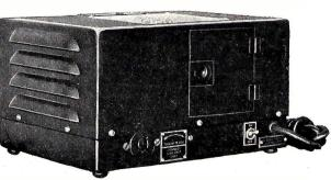
B-L SELENIUM RECTIFIER ASSEMBLY. Output rating 0.5 amperes, 115 volts DC, filtered and regulated. Operates from 115 volts, 50-60 cycles AC. Size 12" x 6" x 8".
