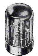
The accelerometer is a newly developed electronic tube useful in measuring linear acceleration. Operating range -1 to 100 g's.
