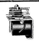
Type F The F relay is a single pole relay for DC particularly adaptable in ap-plications where space is limited. Bakelite insulation is used. May be supplied with other contact combina-tions. Silver is standard contact ma-terial, alloy contacts can be substi-tuted. Contact rating is 3 amperes at 24 volts DC or 115 volts AC non-inductive. Nominal power rating is .750 watts. Weight 1-7/8 ounces. Length 1-3/32". Width 1-3/16". Height 1-11/32". Type F
