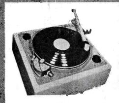
62A Transcription Turntable has been widely used by broadcast stations and recording studios during the past five years. It is rim driven through a machined rubber tire at the outer diameter of the turntable, providing a very simple and quiet drive.
