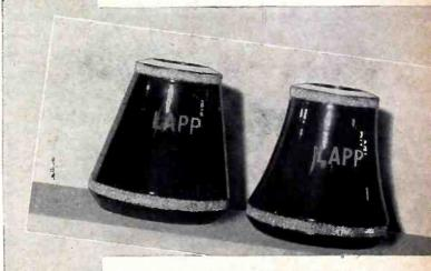
All Lapp footing and guy insulators incorporate the Lapp patented curvedside compression cone {right}. With the same dimension and same wall thickness, the curved-side cone has double the strength of the straight-side cone {left}.
