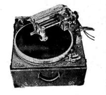
**6N Recorder** (16") has proven ideal for most broadcast stations and recording studios because of its high quality and relatively economical cost. It is supplied in carrying case for portable and remote assignments as well as in a cabinet. Its design is of the conventional rim driven type with overhead feed mechanism.
