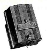
1-D Cutting Head provides stability, uniformity, and sensitivity with low distortion for recording transcriptions having specified, response characteristics such as flat, NAB, etc. Response: 50-10,000 cps. Crossover at 500 cps. Résponse and level not affected more than  $\pm 21/2$ db between 60° and 95° Fahrenheit.
